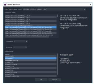
Additionally the behavior supports a Card Id, used to obtain the cards API endpoint address and a Write Mode which can be used to fix the behavior into either Read/Write (or both) modes. In most cases Read/Write won't hurt, even if only using for display purposes, however Read only will be slightly more efficient in these cases.
