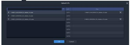
The list of available LUT files can be filtered. Use the drag handle to drag and drop the file into the appropriate slot. Up to eight slots can be populated. After clicking OK the LUT files will be uploaded to the respective slots on the selected devices.
