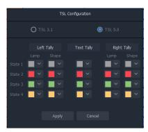
• [Ref. #UCCM-1894] **Ability to Easily Assign TSL Value to Widget:** Added feature to enable the user to quickly assign TSL functionality to Tally Lamp, Label and Shape Widgets. Select the widget, right click and select **TSL configuration**. Select the source of the tally, e.g. left or right tally. Select the TSL address level, e.g. L1, L2 etc. If the user has renamed the levels then their custom labels will be shown.
