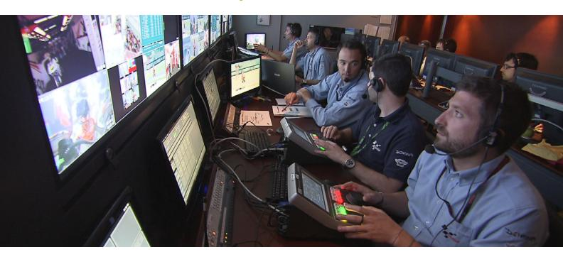
Each of Dorna's eight K2 Dyno Replay Systems consists of a K2 Summit™ media server and a K2 Dyno Replay Controller, which allows each operator to mark and tag clips, cue up replays, and play them back, using variable speed and mix effects to add production value.
