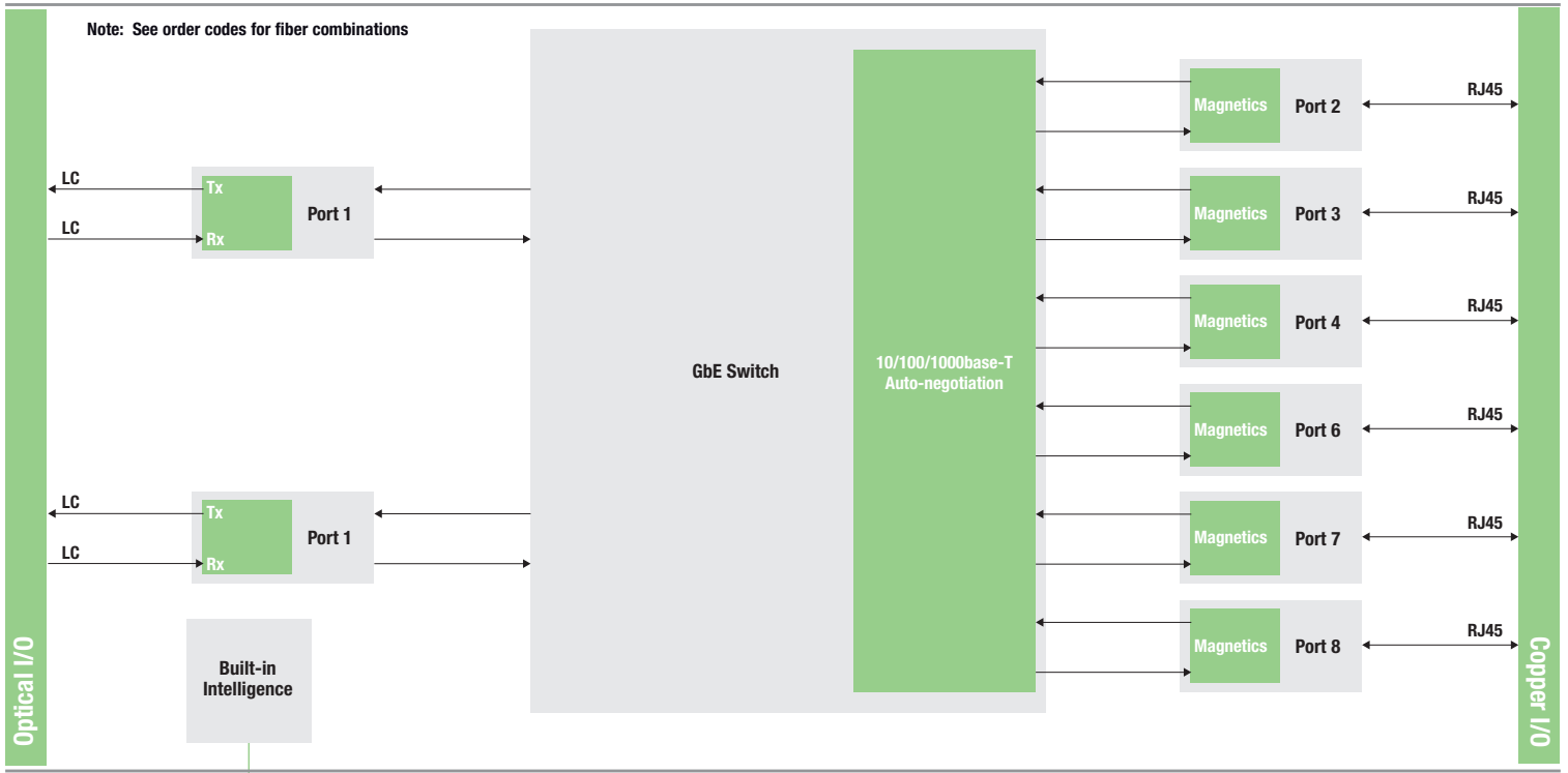
Block Diagram for IQGBE8000-2B.
