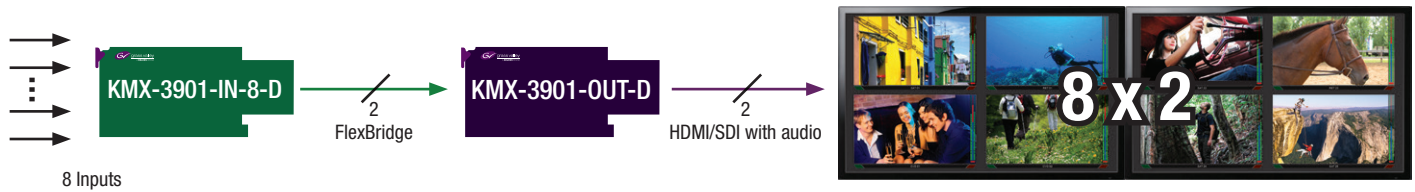
8 x 2 configuration using one KMX-3901-IN-8-D and one KMX-3901-OUT-D
