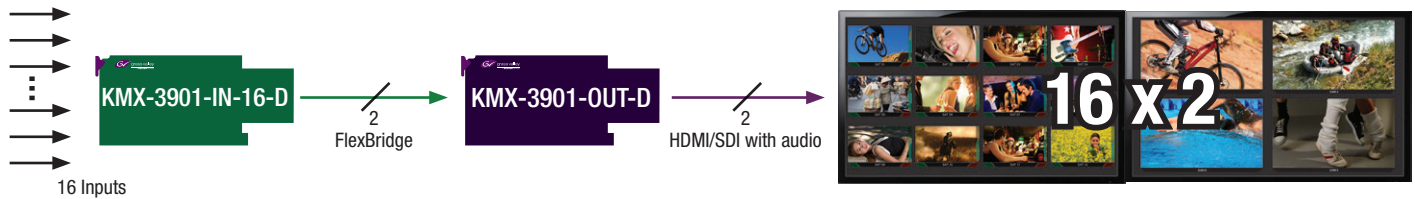
16 x 2 configuration using one KMX-3901-IN-16-D and one KMX-3901-OUT-D
