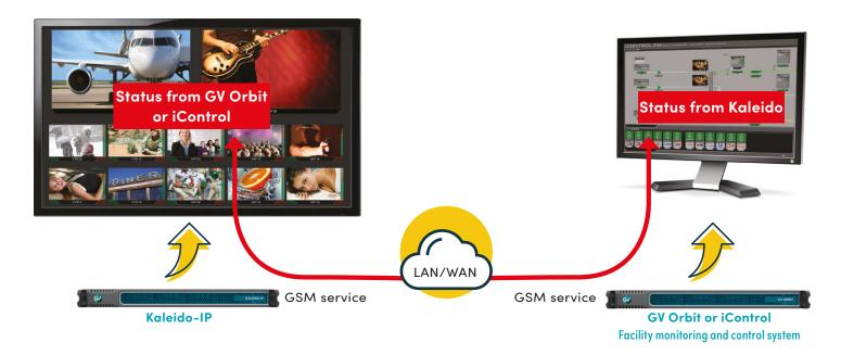
GV Orbit's or iControl's extensive library of third-party devices allows Kaleido-IP to leverage existing IP and MPEG probing devices to increase alarming capabilities.
