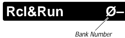
Figure 4-7. Auto Run Display, Bank 0 Selected
