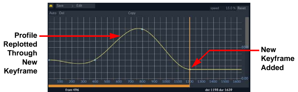
Figure 77 Keyframe Node Inserted into Respeed Profile
