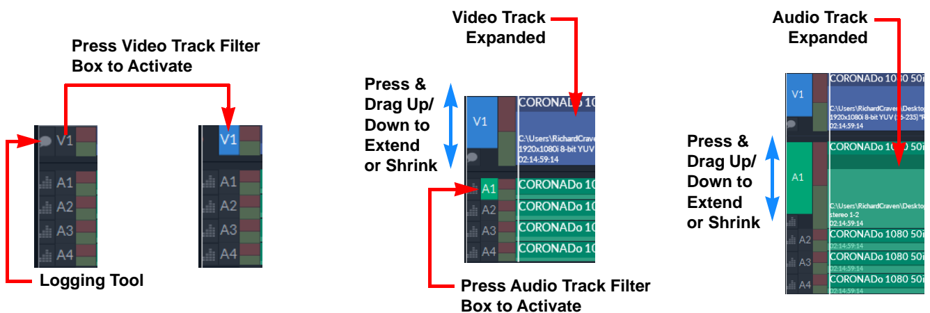
Figure 21 Scaling Audio & Video Tracks in a Floating Clip Using the Track Filters
