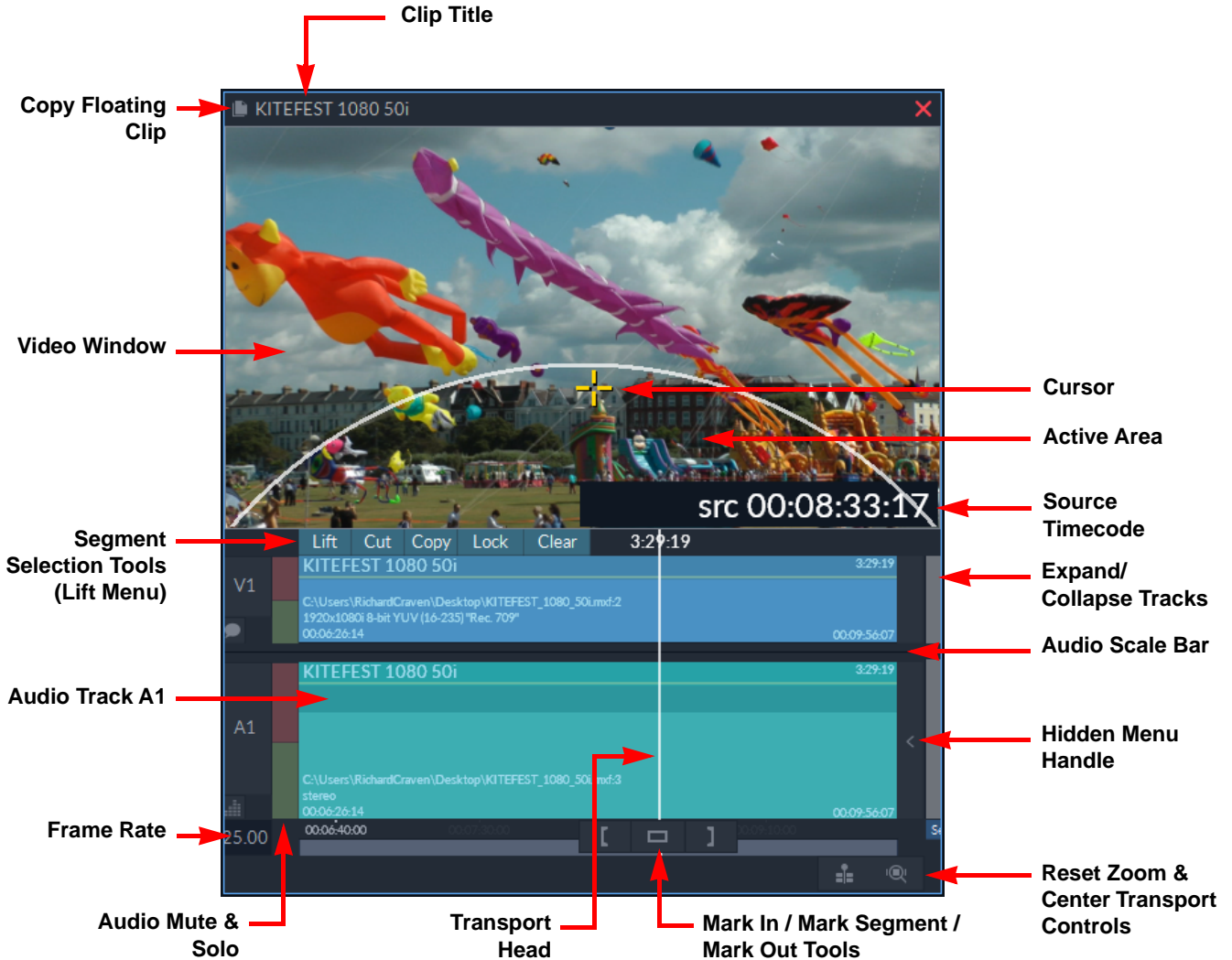
Figure 15 Overview of a Floating Clip Panel
