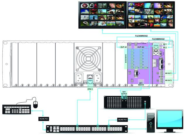
Typical Cabling diagram, showing rear view of a Kaleido-Modular-X  $16 \times 2$  system
