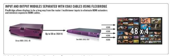
Kaleido-Modular-X distributed configuration with 48 inputs and 4outputs
