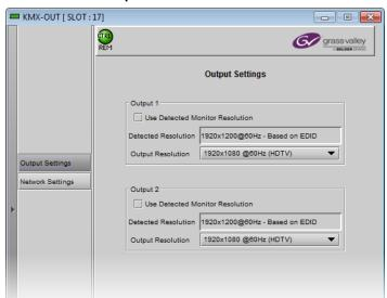
The following table lists some (but not all) output formats supported at the HDMI connections. You can customize your own timing rates for resolutions ranging from  $1024 \times 768$  pixels up to  $1920 \times 1200$  pixels (all progressive scan), by using XEdit.
