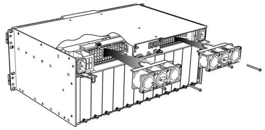
3 Use the two screws you retained from the old fan, to secure the new fan assembly to the rear panel.
