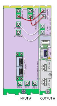
FlexBridge wiring for a 12 × 2 IP system
