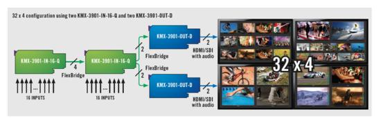
Kaleido-Modular-X configuration with 32 inputs and 4 outputs
