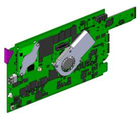
Note: Output cards with a single rear connector panel (KMX-3901-OUT-D-3+SRP) are compatible with Densité 3+ FR1, and Densité 3+ FR4 only.
