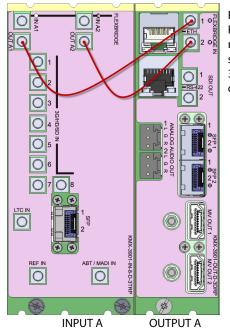
Rear panels for a KMX-3901-IN-8-D (left), and KMX-3901-OUT-D (double panel shown on right). The Flexbridge connectors are the same on the KMX-3901-IN-8-D and KMX-3901-IN-16-D card's rear panels, and on the output card's single and double rear panels.
