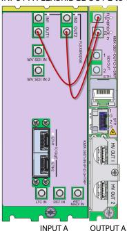
Rear panels for a KMX-3901-IN-IP-D (left), and KMX-3901-OUT-D (single panel shown on right). The Flexbridge connectors are the same on the KMX-3901-IN-8-D and KMX-3901-IN-16-D card's rear panels, and on the output card's single and double rear panels.
