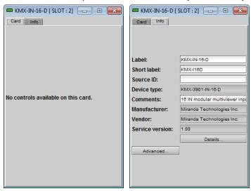
Service control panel for a KMX-3901-IN input card
