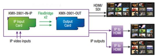
Kaleido-Modular-X configuration with IP inputs, 2 IP outputs, and 2 HDMI/SDI outputs
