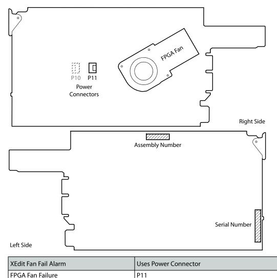
The location of the fan on the KMX-3901-OUT card is shown below.
