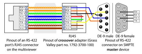
Standard wiring between multiviewer and devices wired to SMPTE "master" specification (e.g. Philips Jupiter router control system, Grass Valley Presmaster PCS)
