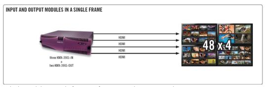
Kaleido-Modular-X single-frame configuration with 48 inputs and 4 outputs
