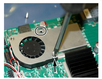
Once the 2 screws are removed, remove the fan cover assembly.
