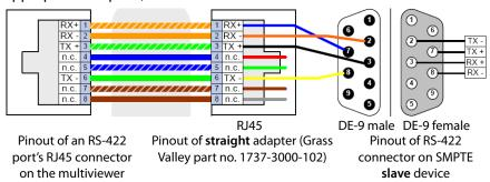
Standard wiring between multiviewer and devices wired to SMPTE "slave" specification (e.g. most routers, Ross Synergy switchers, Nevion ETH-CON)
