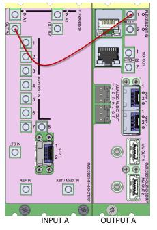
Rear panels for a KMX-3901-IN-8-D (left), and KMX-3901-OUT-D (double panel shown on right). The Flexbridge connectors are the same on the KMX-3901-IN-8-D and KMX-3901-IN-16-D card's rear panels, and on the output card's single and double rear panels.
