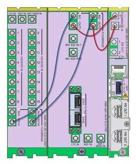
Rear panels for a KMX-3901-IN-16-D (double panel shown on the left), KMX-3901-IN-IP-D (center), and KMX-3901-OUT-D (single panel shown on the right). The Flexbridge connectors are the same on the KMX-3901-IN-8-D and KMX-3901-IN-16-D card's rear panels, and on the output card's single and double rear panels.
