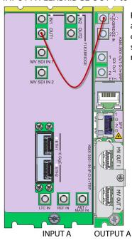
Rear panels for a KMX-3901-IN-IP-D (left), and KMX-3901-OUT-D (single panel shown on right). The Flexbridge connectors are the same on the output card's single and double rear panels.
