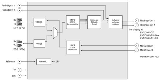
Kaleido-Modular-X functional block diagram: KMX-3901-IN-IP input/output modules
