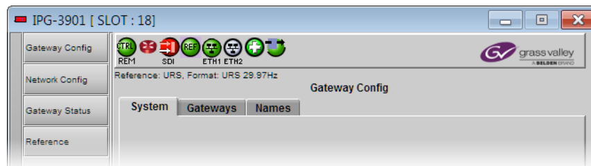
Service control panel for an IPG-3901 gateway card—partial view showing status icon area
