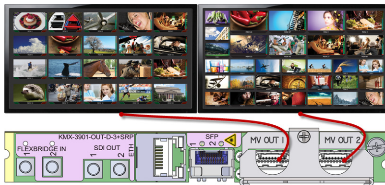
HDMI outputs on single rear module, connected to displays
