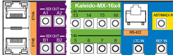
System control connectors on Kaleido-MX 4K 16 × 1
