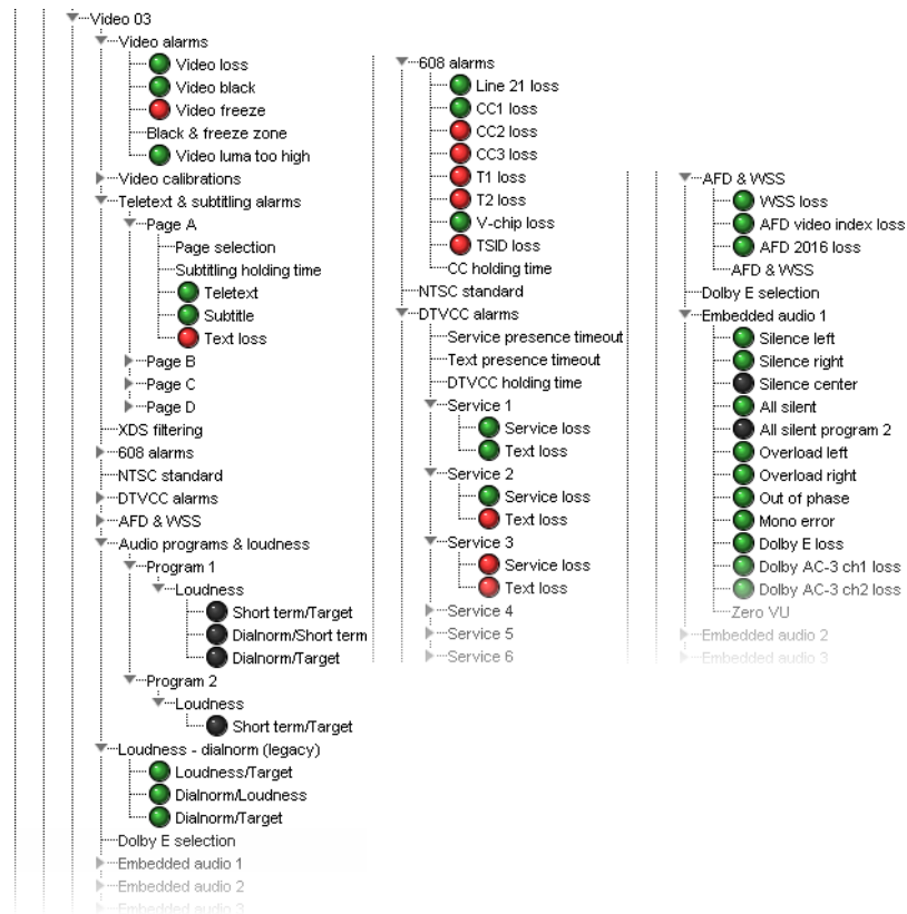
Example of alarms related to video and embedded audio input signals, for Kaleido-X, Kaleido-X16, and KMV-3901/3911 multiviewers.
