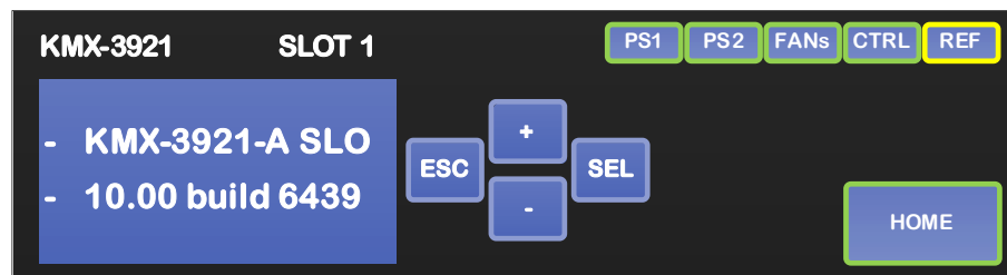
CPU-ETH3 local control panel
