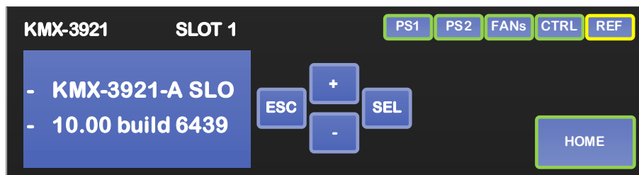
CPU-ETH3 local control panel
