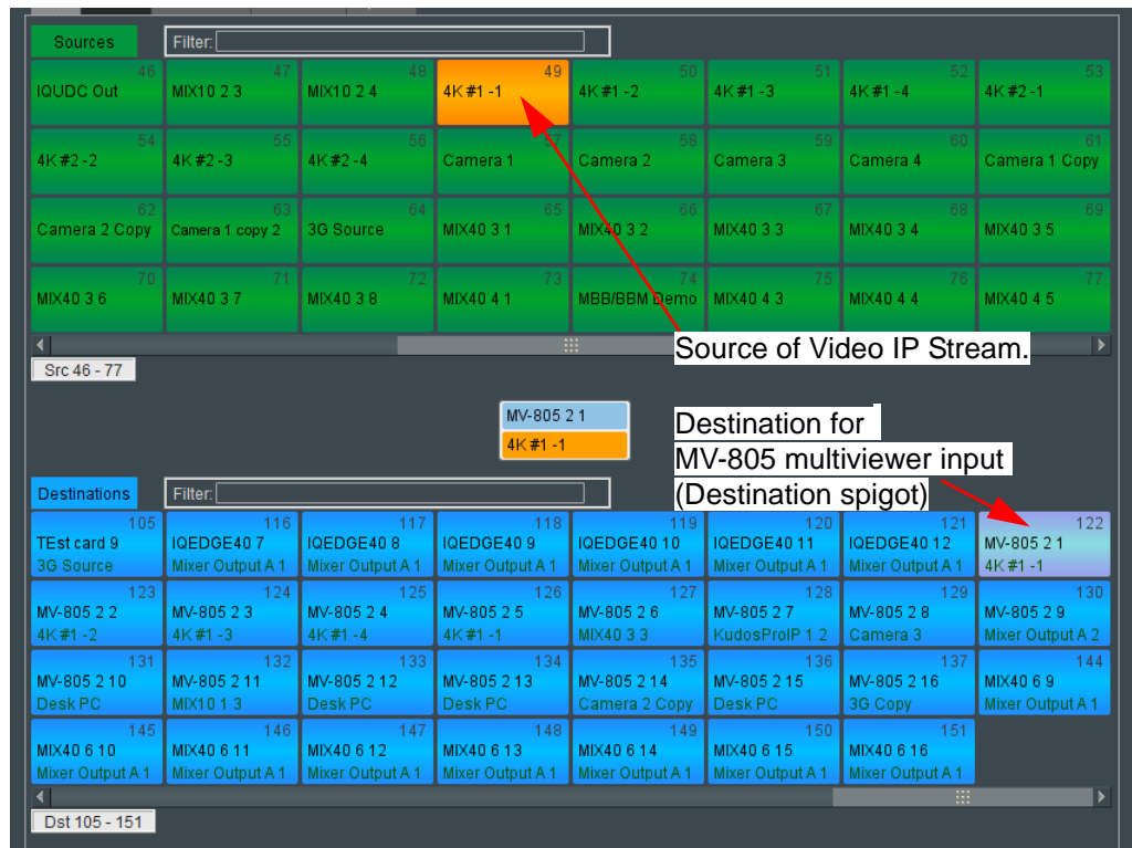
Figure 88 Multicast Video IP Stream Routed to an MV-805 Multiviewer Input
