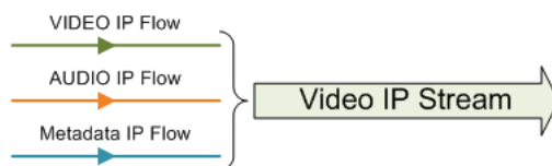
Figure 5 IP Flows comprising a Video IP Stream
