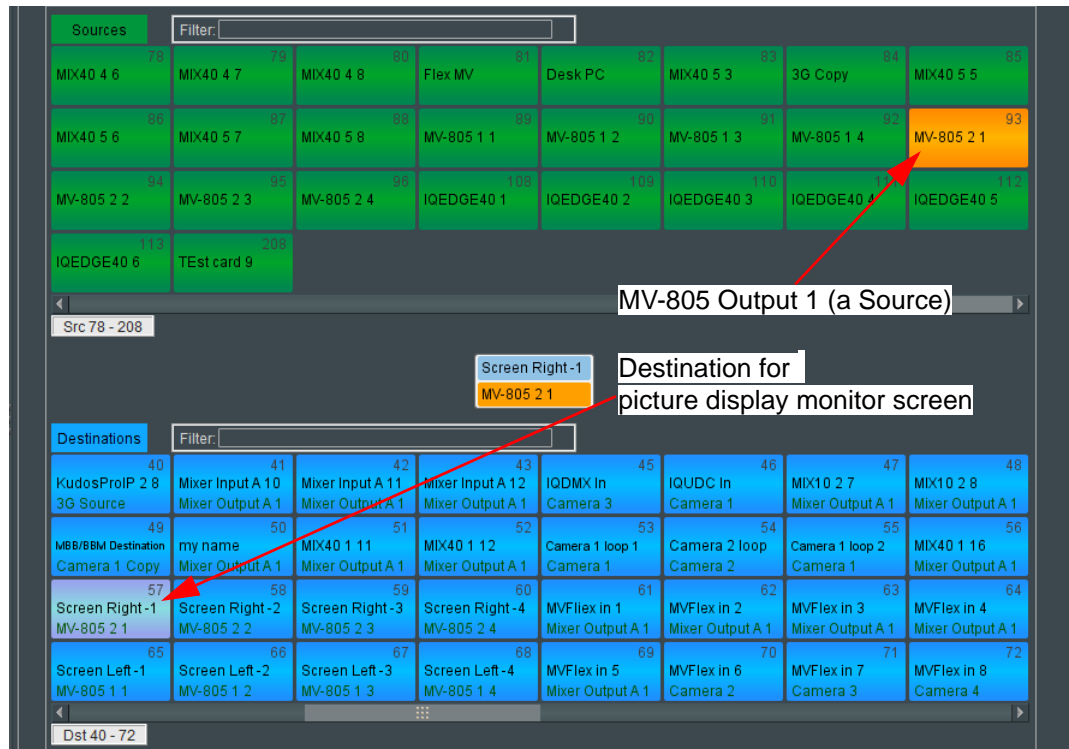
Figure 87 MV-805 Display Output Routed to a Display Monitor
