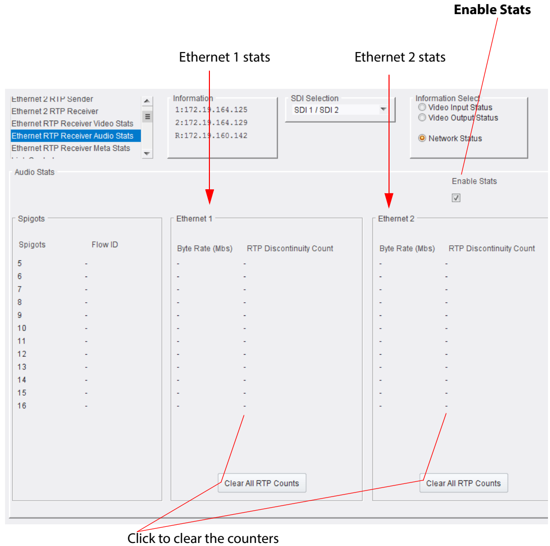
Figure 63 Ethernet RTP Receiver Audio Stats Template
