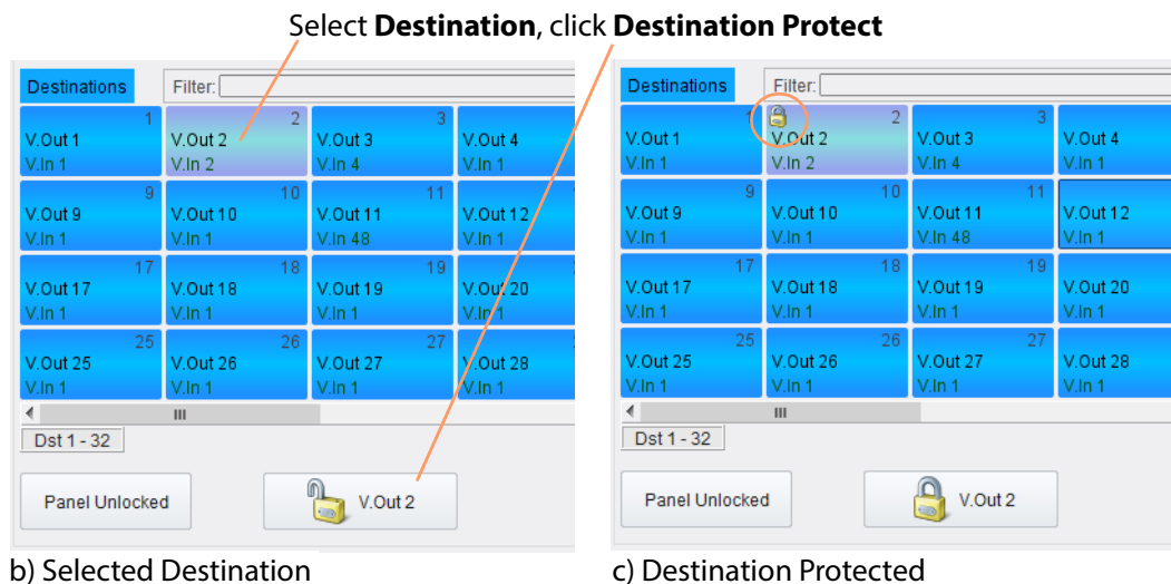
Fig. 6-7: Destination Protect (Lock Route) a) Not Locked/Protected; b) Selected Destination; c) Destination Protected
