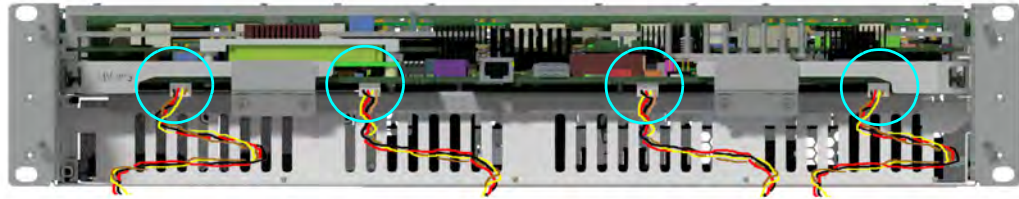
Fig. 2-4: Fan Supply Wires Connected to front of the Main Card
