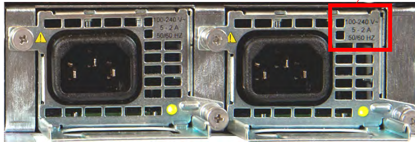
Rear Mains Inlets and Mains Supply Rating
