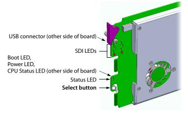
The Status LED on the selected card flashes orange, and the associated control menu appears on the display of the Densité frame's local control panel.
