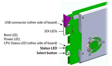
The Status LED on the selected card flashes orange, and the associated control menu appears on the LCD display of the Densité frame's local control panel.
