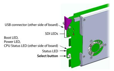
The Status LED on the selected card flashes orange, and the associated control menu appears on the display of the Densité frame's local control panel.
