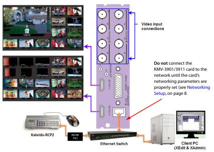
Cabling diagram (showing KMV-3911 rear panel)
