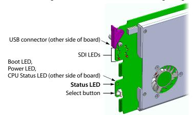
Once the startup has completed, the Status LED should be red (steady) because the card is not connected to the network yet:
