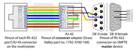
Standard wiring between multiviewer and devices wired to SMPTE "master" specification (e.g. Philips Jupiter router control system, Miranda Presmaster PCS)
