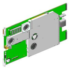
The KXO-Dual and KXO-Dual3 are multi-function cards that perform a significant portion of the signal processing required to create the monitor wall output. They incorporate a mezzanine card mounted on the component side. Each output card is complemented by a rear panel (KXO-Dual-R) that holds all input and output connectors associated with the card.
