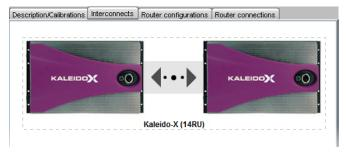
When two frames are joined, the default names for all available inputs are formed by concatenating the frame name, the input card, and the video number. For example, the logical source "/Frame A/Input C/Channel 01" corresponds to the first video input on KXI card C on Kaleido-X **Frame A**.
