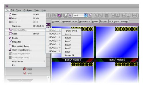
The **Copy layout to** window opens, displaying the currently open layout on the left, and the target layout on the right.
