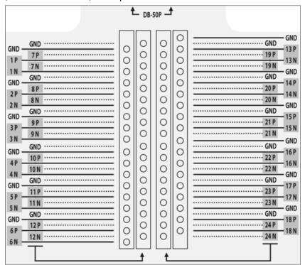
Adapter are not used as connections. Positive pins (labelled with a P) and Ground pins (labelled with a GND) correspond to GPI-IN connections.
