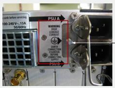
Connect a ground cable between this stud and the rack
