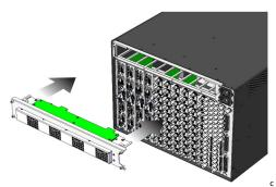
Installing fan assembly into KXA-FR7-B frame model
