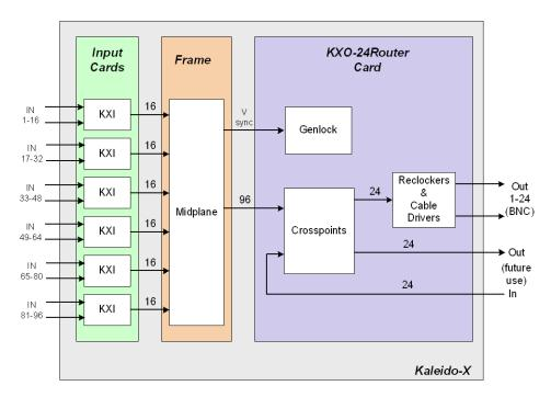
Simplified Signal Flow Diagram - KX0-24Router
