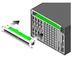
Installing fan assembly into KXA-FR7 frame model
