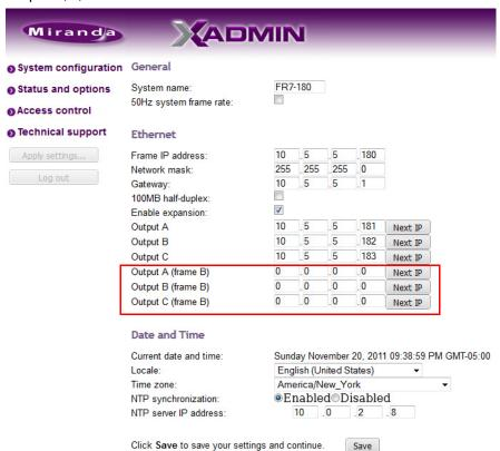
The Output D/EXP IP address is replaced with new lines for the IP addresses of Frame B's Output A, B, and C cards.
