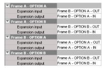
All sources can now be routed to any internal router destination via the router expansion cables.
