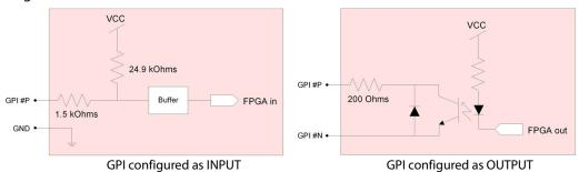
You should ensure your GPI physical connections are well established. In the following example, the goal is to trigger a relay and light up a light.
