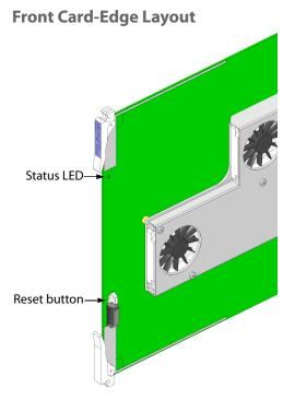
A single LED status indicator is visible on the front edge of the card:
