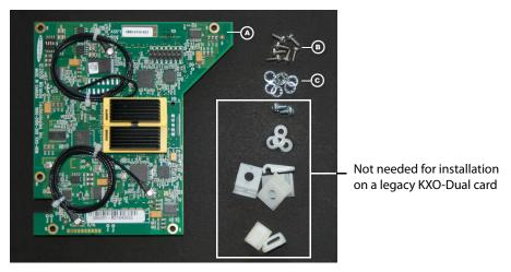
Before you start, make sure that you have a Phillips #1 screwdriver at hand, and that you are wearing a static control wrist strap. Allow approximately 15 minutes to complete the installation.
