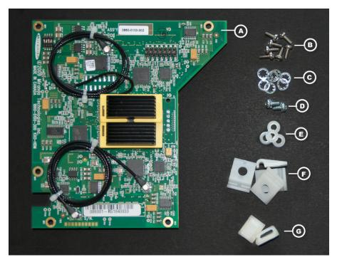
Before you start, make sure that you have the Phillips #1 screwdriver, and long nose flat pliers needed to perform this installation, and that you are wearing a static control wrist strap. Allow approximately 20 minutes to complete the installation.
