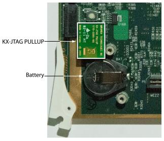
The mezzanine is installed in the lower left corner of the card.
