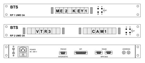
Connection to the MPK bus is made in the same way as for the AUX panels. Power supply can be universally with line voltages of 85 V  $\dots$  265 V AC. The respective use of the UMDs can be adjusted with the two rotary switches **ADDRESS** on the terminal panel.
