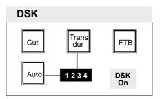
CutCut performs the transition as a hard cut.AutoAuto performs a transition with the preset transition rate.<br/>The key will light for the duration of the transition and the selected transition rate<br/>is shown in the display. Pressing the Cut key completes the transition instanta-<br/>neously.<br/>If the automatic transition has been started erroneously, it can be stopped and can-<br/>celled by pressing the Auto key again.<br/>Keying-in with DSK is indicated by the DSK On display.
