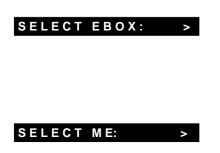
In the sub-loop all E-Box types in the network can be indicated and then be selected with **Edit**. A selected E-Box is marked with an aster-isk.
