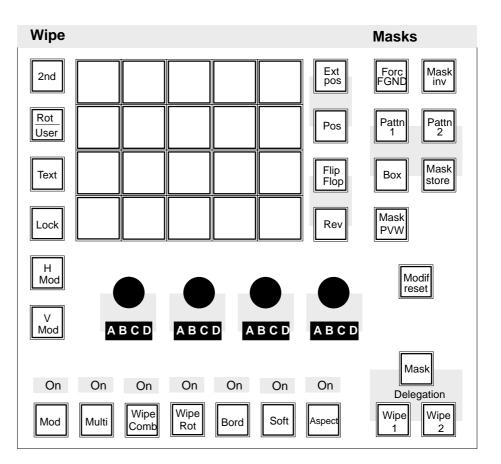
By means of the modifier keys **Mod**, **Multi**, **Wipe Comb**, **Wipe Rot**, **Bord**, **Soft** and **Aspect**, the standard wipe patterns can be changed and even new patterns can be created by combinations of patterns.
