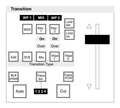
For picture design, selection can be made between the transition modes *Add*, *Mix*, *DVE*, and *Wipe*, providing up to two wipe generators. The individual picture components can be simultaneously faded with different transition types.
