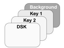
Beside the main outputs, the switcher additionally includes a clean-feed output which provides the picture in front of the downstream keyer.
