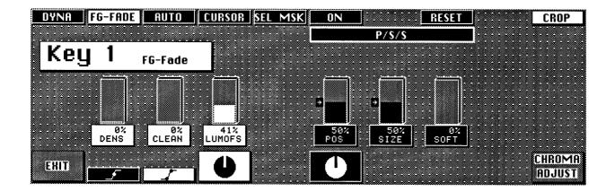
LUMOFS positive luminance offset to the subtractive key color luminance (only in the FG Fade mode). Raises or lowers the luminance level in the transition areas. Can be used in order to brighten too dark object edges or to darken too bright edges, for better matching them to the background scene.
