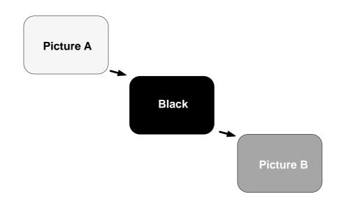
Transition can be made with Cut, Auto or manually with the fader.
