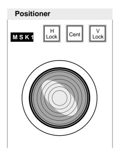
*H Lock, V Lock* **H lock** and **V lock** permit locking the trackball in H or V direction. Thus, it is possible, for instance, to exactly position a wipe pattern along a horizontal or vertical line.
