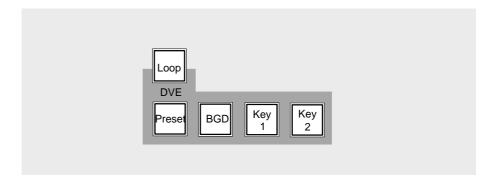
If **Loop** is not actuated, the respectively selected video signal is switched through to the DVE. The manipulated signal of the DVE is available on the input routing switcher and can be processed in the same way as a normal video signal.
