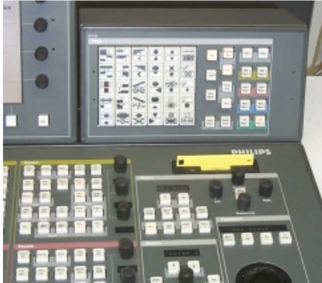
Fig. 203: Floppy disk drive in the RPS35-4 panel
