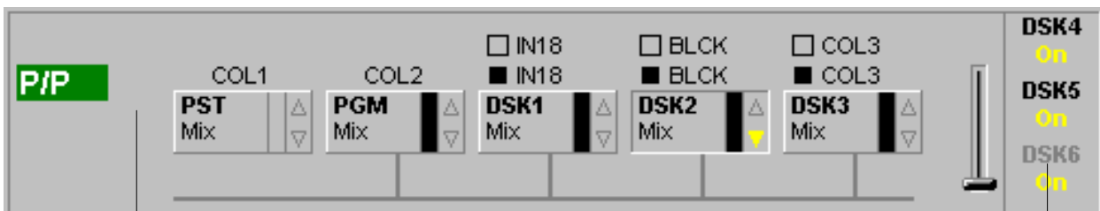
Example 4 Status display of the mixing level P/P, always “non-layered / key3 mode” .
