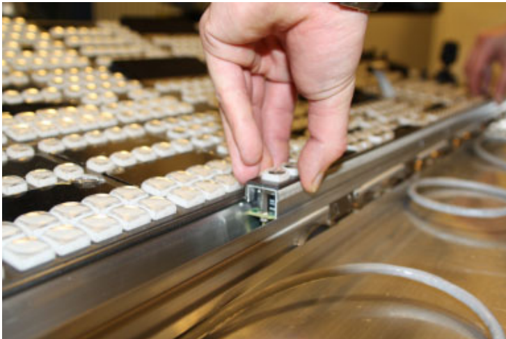
Aligning the System Bar for Replacement
