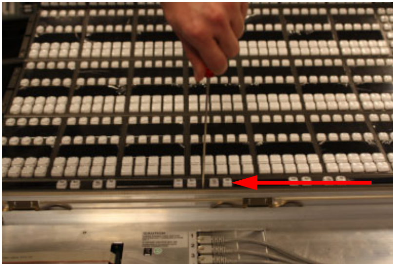
Unscrewing the System Bar
