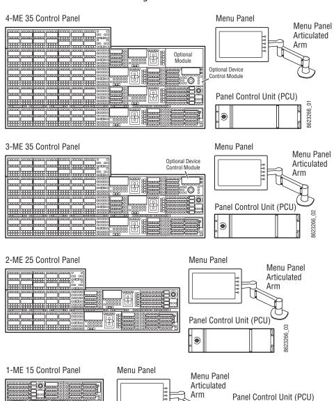
Panels. This control surface has an innovative modular design. Representative Kayenne control surfaces are shown in the following illustrations.
