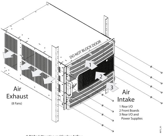
8-RU Rack Mounting and Cooling Airflow
