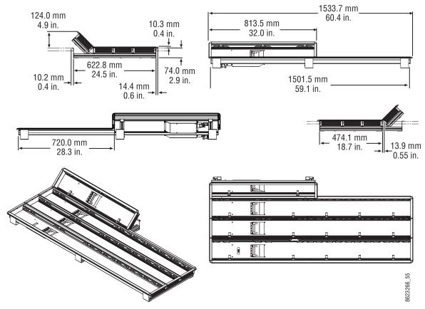
3-M/E 35 Control Panel Dimensions, Flat Installation
