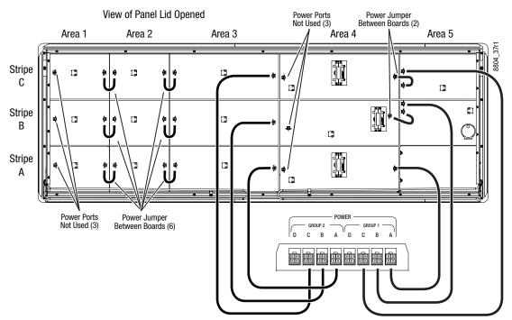
Power Cable Internal Connections, 3-ME Panel
