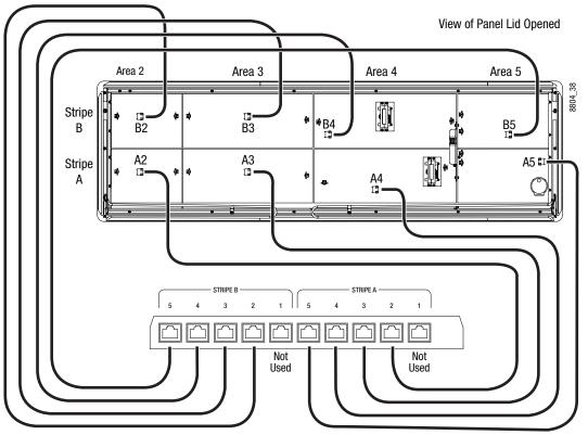
Data Cable Internal Connections, 2-ME Panel
