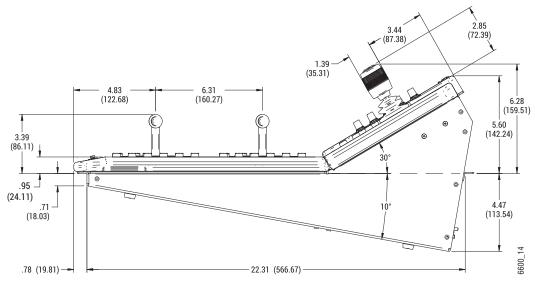
2-M/E GV Korona Control Panel Mounting Dimensions
