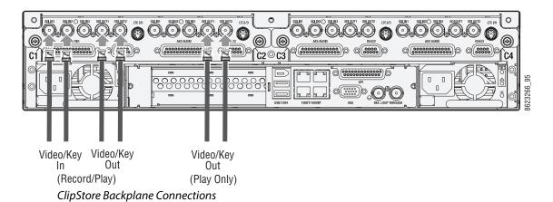
The ClipStore server (4-channel Summit/2-Channel Solo) can be connected directly to the frame. It is also possible to connect to the ClipStore directly from a router and not use any switcher outputs.
