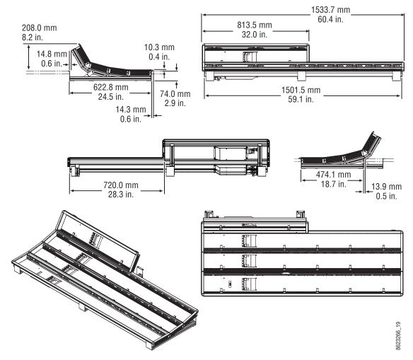
3-M/E 35 Control Panel Dimensions, Curved Installation
