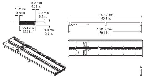
2-M/E 35 Control Panel Dimensions, Flat Installation
