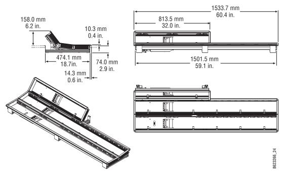
2-M/E 35 Control Panel Dimensions, Curved Installation
