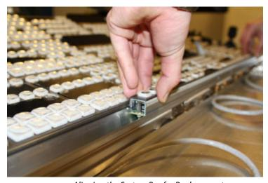
Aligning the System Bar for Replacement
