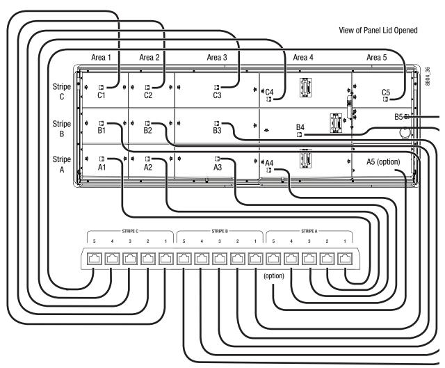
Data Cable Internal Connections, 3-ME Panel
