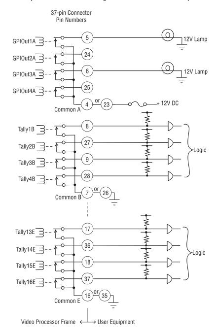
Relay Tally and GPI Output Connection Example
