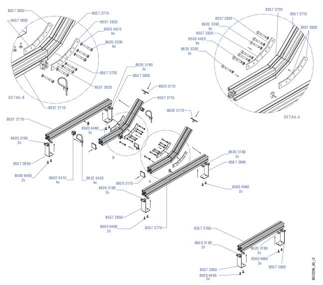
2-M/E Support Structure, Flat Installation
