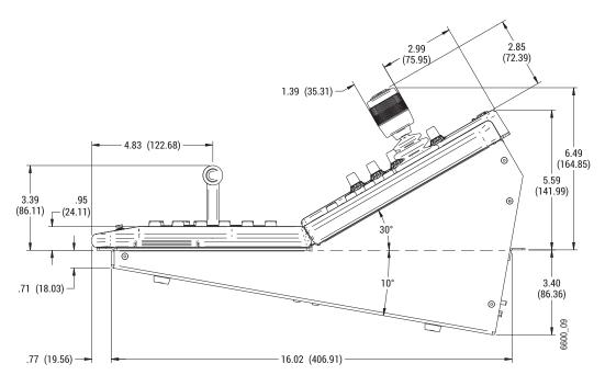
1-M/E GV Korona Control Panel Mounting Dimensions
