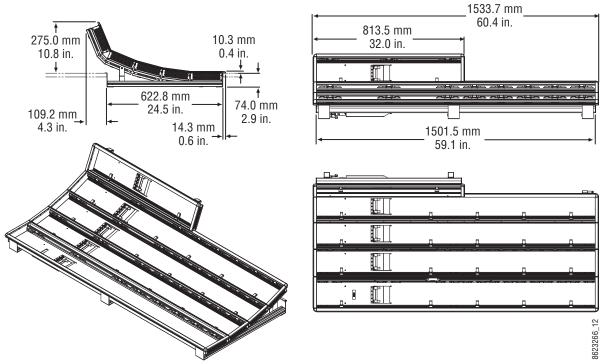
4-M/E 35 Control Panel Dimensions, Curved Installation
