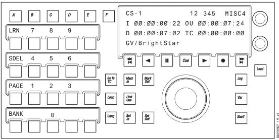
Device Control Module Example
