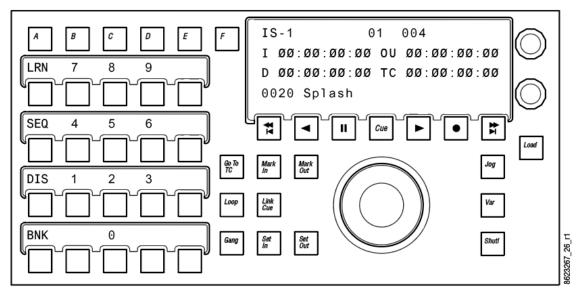
Image Store Device Control—Device Control Module
