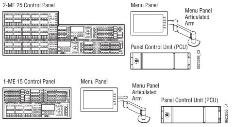
The modular design and use of a separate PCU supports the hot-replacement of individual Control Panel components, if necessary, while the rest of the system remains operational.
