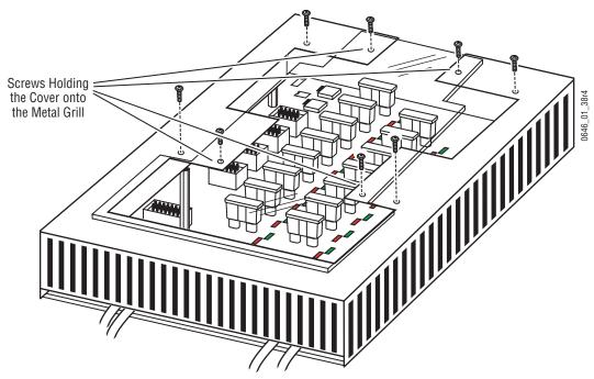
**3.** Remove and replace the fuse and then replace the cover.
