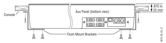
Figure 105. Local Aux Panel Console Flush Mount
