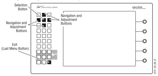
Figure 159. Original Menu Panel Screen Adjustment Control Buttons
