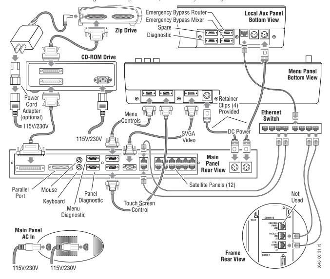
Figure 117. Early Model 4-M/E Control Surface Cabling
