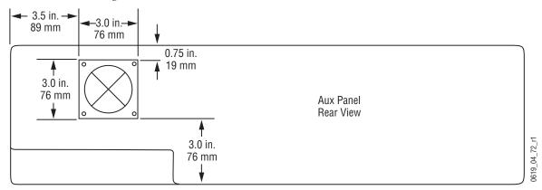
Figure 106. Local Aux Panel Fan Position
