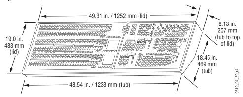
Figure 70. 2-M/E Rear Panel Dimensions
