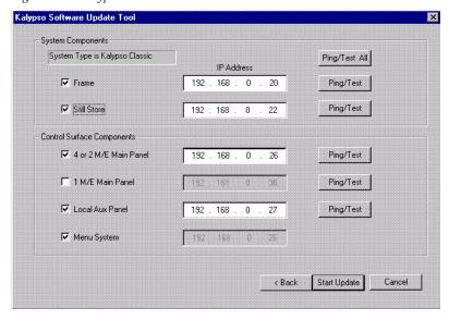
**4.** Touch the **Ping** button for the Main panel, then touch the **Ping** button for the Frame. A message informs you whether each device is responding.
