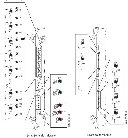
Figure 216. Sync Generator and Crosspoint Module LEDs
