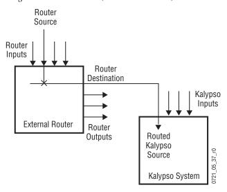
An external router can be configured into levels, to allow the switching of multiple signals simultaneously. For example, video signals can be organized on one level, and key signals on another. By specifying both levels when giving a router take command, both the video and key signals of a source will be routed to their destinations.
