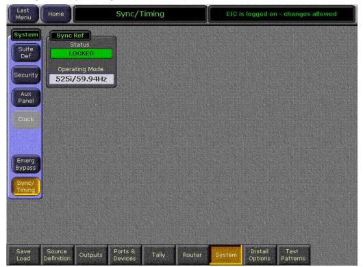
The Kalypso sync regenerator locks to an incoming reference signal and reports the line standard it is regenerating in the Operating Mode field. That operating mode persists until a reference input different from the current line standard is detected and locked to. If the reference signal is temporarily lost, the Kalypso system will continue to free run in that line standard and a NO INPUT status will be reported.
