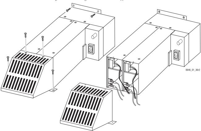
Figure 174. Removing Main Panel Power Supplies
