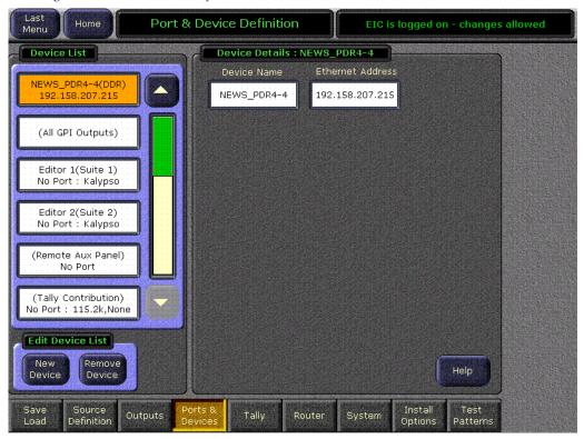
The currently configured device definition objects are displayed in a scrolling list on the left. Touching a device on this list delegates the rest of the menu to that object.
