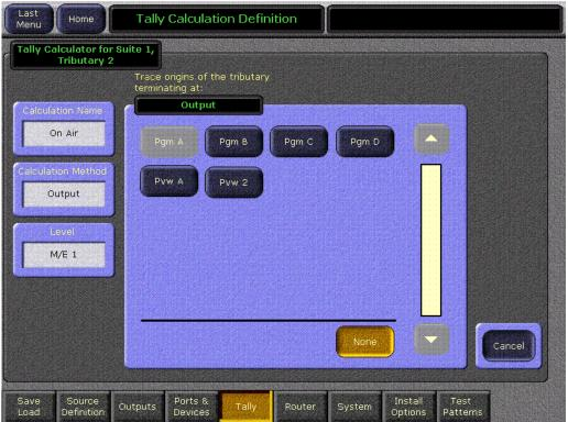
If the Calculation Method is Look Ahead, Aux is grayed out in the Level pane, because there is no look ahead point on an aux bus. Then when a Tributary data box is touched, the following popup in Figure 147 appears.
