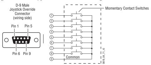
Once installed, the joystick override inputs can be mapped to specific Remote Aux panel buttons. See *Joystick Override* on page 186 for more information.
