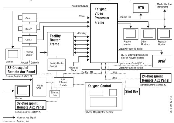
Figure 37. Basic Live Production Studio System Configuration Example
