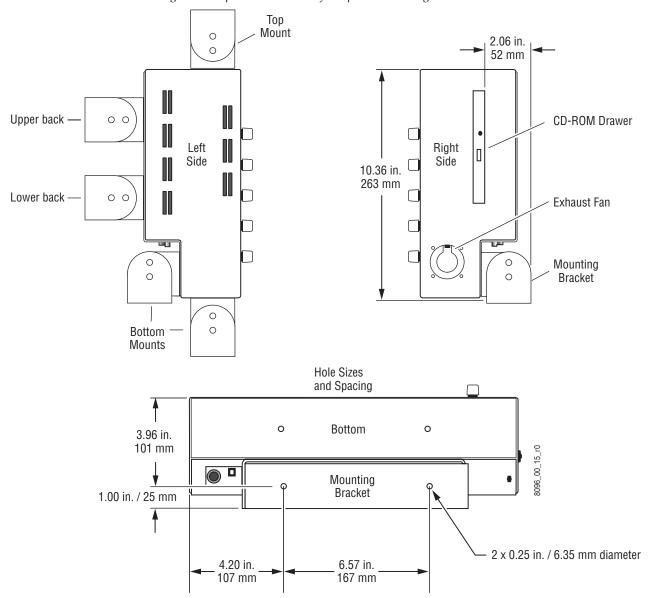
Figure 95. Optional Placement of Adaptable Mounting Bracket
