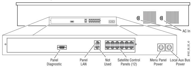
Figure 4. Late Model 4-M/E Main Panel, Rear View
