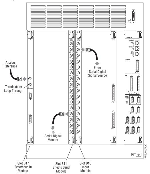
Figure 52. Bench Test Video Connections
