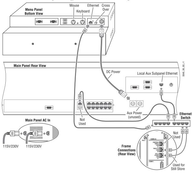
Figure 45. Kalypso 2-M/E Bench Test Ethernet Cabling
