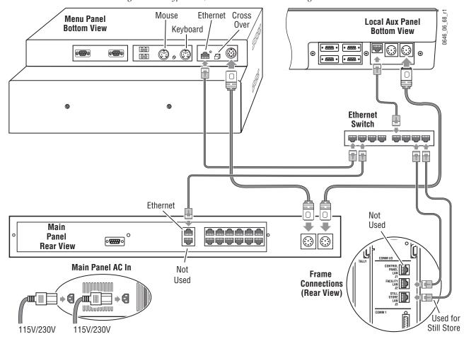
Figure 44. Kalypso 4-M/E Bench Test Ethernet Cabling
