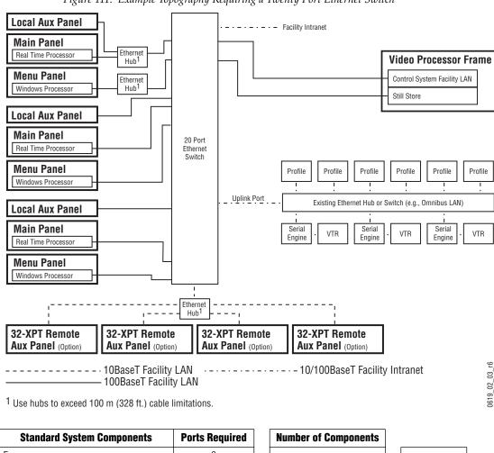
Figure 111. Example Topography Requiring a Twenty Port Ethernet Switch
