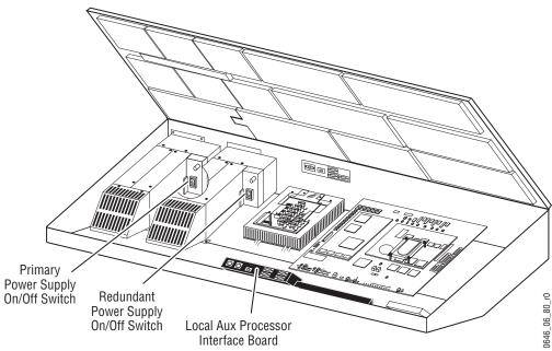
Figure 170. Local Aux Processor Interface Board Location
