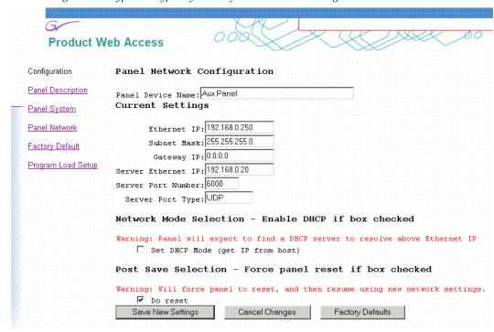
Figure 129. Typical Kalypso System Default IP Address Settings
