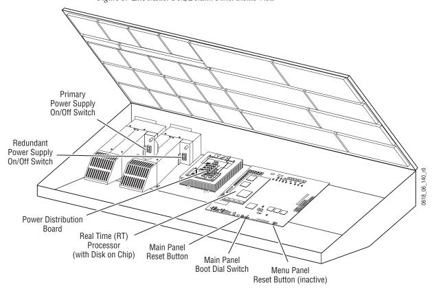
Figure 5. Late Model 4-M/E Main Panel Inside View
