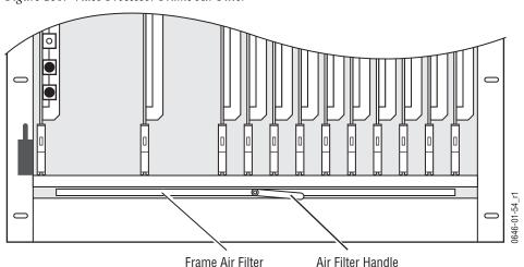
Figure 160. Video Processor Frame Air Filter
