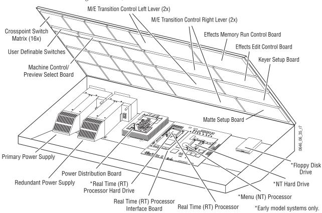
Figure 212. 4-M/E Main Panel Interior Circuit Boards
