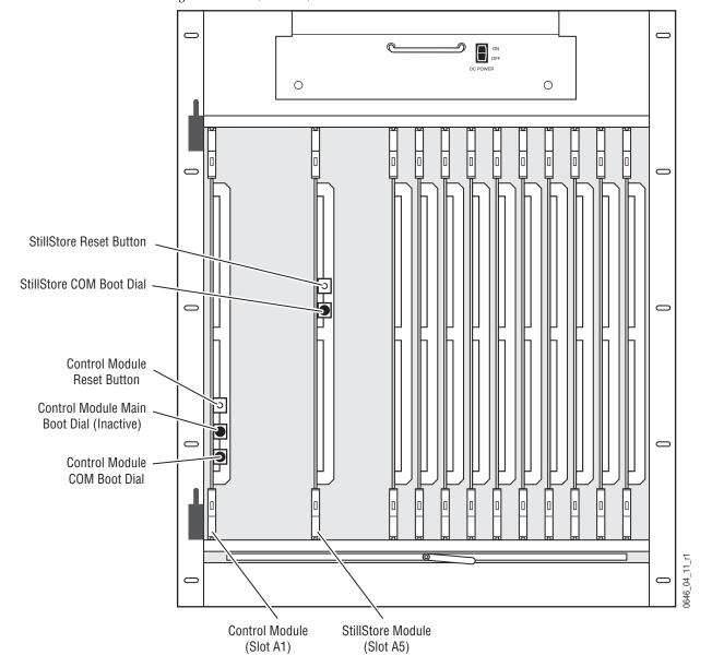
Figure 207. 4-M/E Frame, Front View
