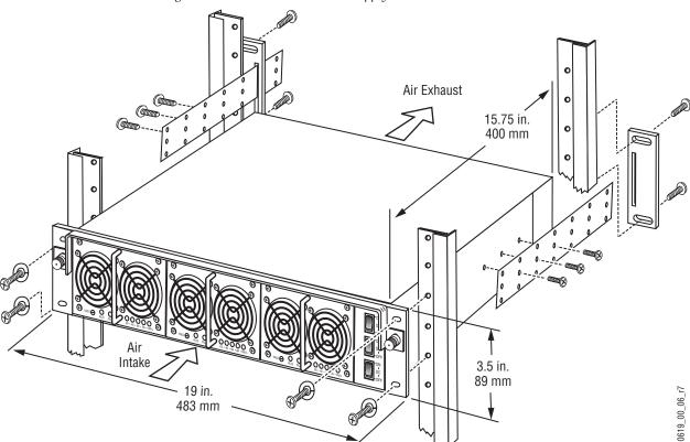
Figure 59. Video Processor Power Supply Installation
