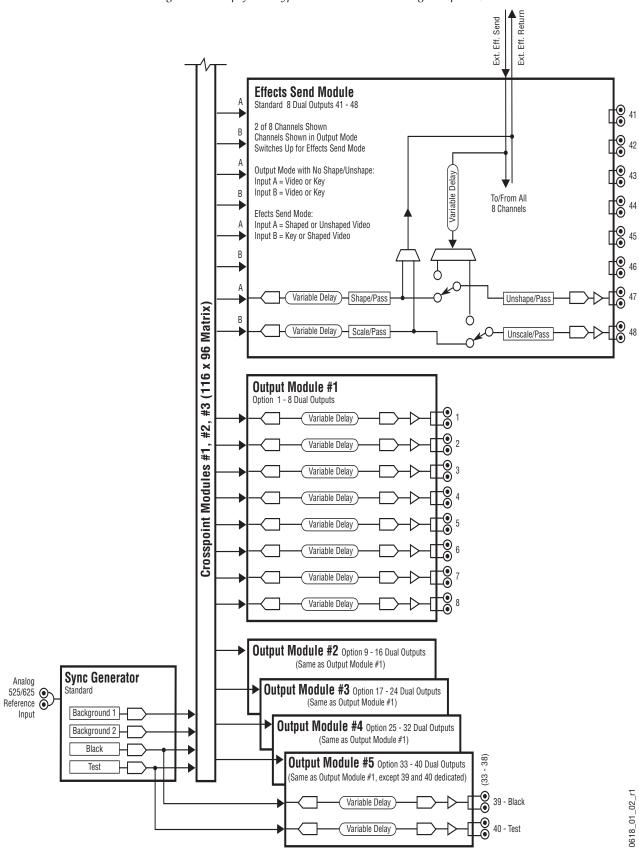
Figure 43. Simplified Kalypso Classic Video Flow Diagram (part 2)
