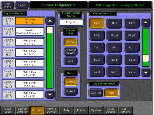
The scrolling list of data pads along the left side of the screen shows the currently assigned output for each listed module connector pair. The scrolling list on the right side shows the available outputs.
