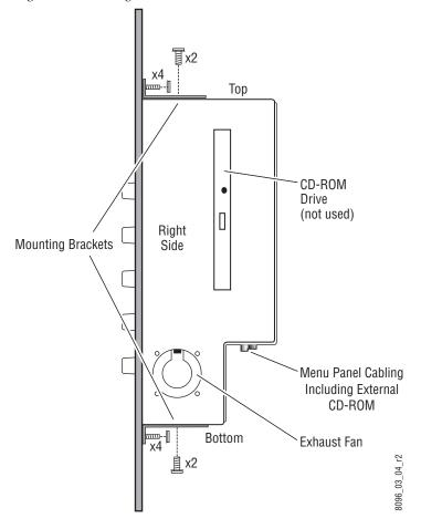
Figure 98. Attaching Flush Mount Bezel to Menu Panel
