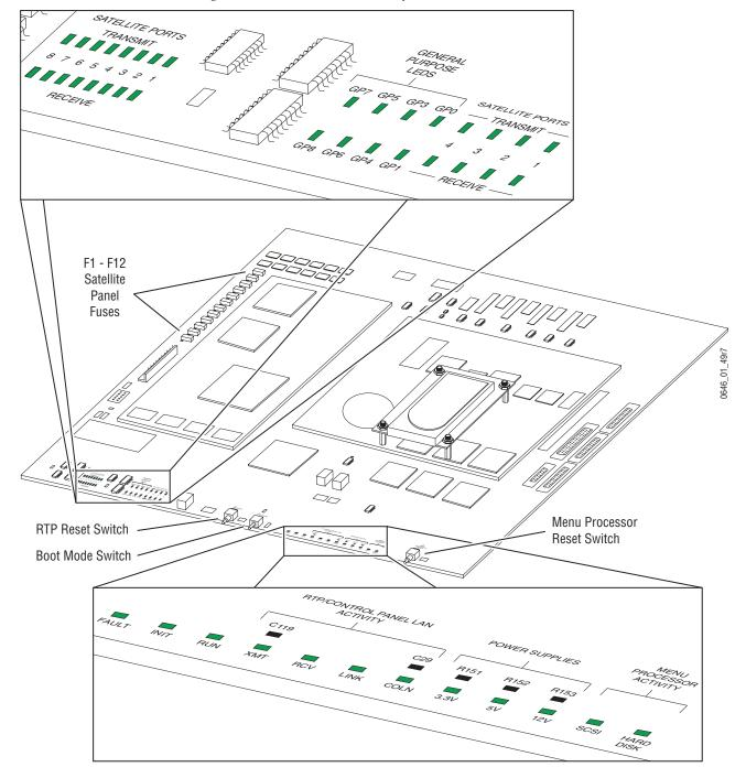
Figure 211. Real Time Processor Interface Board Status Indicators
