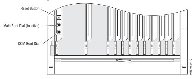
Figure 197. Main Panel Boot Dial Switch
