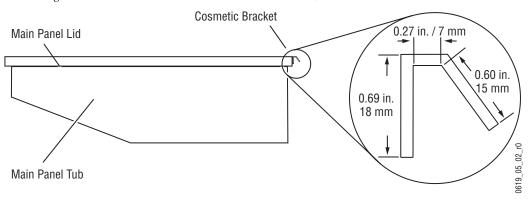
If you choose to use the cosmetic bracket and your Main panel installation has a console support structure similar to that shown in Figure 65, it will be necessary to cut notches in the support members at the left and right rear corners of the console cutout (see the notch dimensions in Figure 65). This enables the Main panel lid to clear the support structure upon opening.
