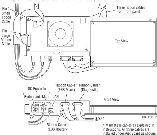
Figure 171. Local Aux Processor Interface Board Cabling
