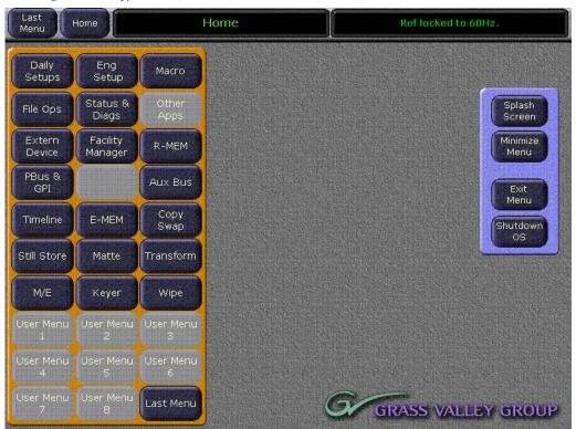
**18.** Touch the **Status & Diags** button to go to the Versions menu (Figure 48). The software reported for each system component should be the latest version, and all the versions should be the same (if the Still Store option is not installed its version will be blank). This confirms the correct Kalypso software is loaded on all system components.
