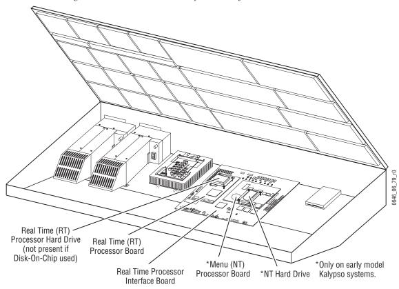
Figure 169. Real Time Processor Interface Assembly
