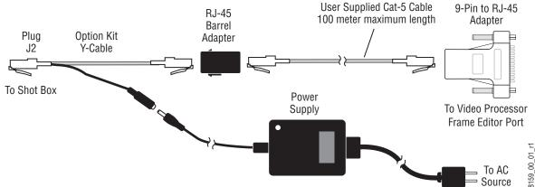
The default Video Processor frame editor port is J11, but a different port can be configured if desired using the Eng Setup Port & Device Definition menu.
