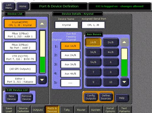
Figure 210. Eng Setup - Port & Device Definition Menu
