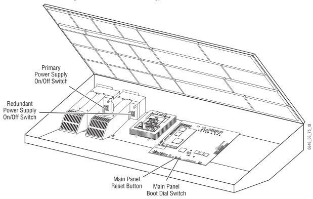
Figure 186. Late Model 4-M/E Kalypso Main Panel Reset Switches
