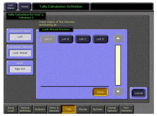
If the Calculation Method is Bus Selection, and if the Level is M/E 1, M/E 2, M/E 3, or Pgm-Pst, and the user touches a Tributary data box, the following popup in Figure 148 appears. All the input buses in the M/E are shown, and the key buses are shown as separate Video (fill) and Key (cut) buses.
