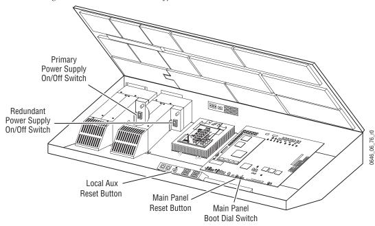
Figure 187. Late Model 2-M/E Kalypso Main Panel Reset Switches
