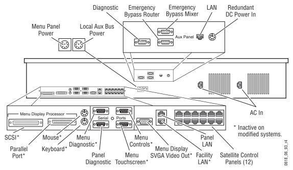
Figure 18. Early Model 2-M/E Main Panel, Rear View
