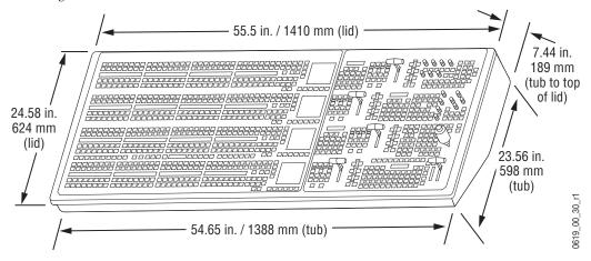
Figure 67. 4-M/E Rear Main Panel Dimensions
