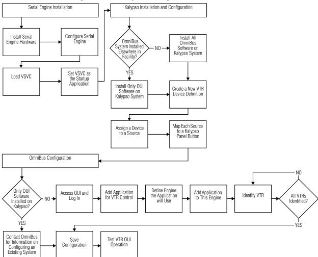
Figure 233. VTR Interface Flow Diagram
