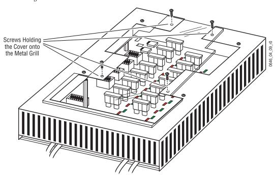
Figure 199. Power Distribution Board
