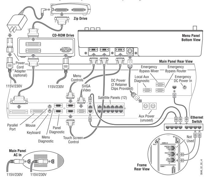
Figure 118. Early Model 2-M/E Control Surface Cabling
