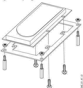
Figure 168. Replacing Board Mounted Hard Drives
