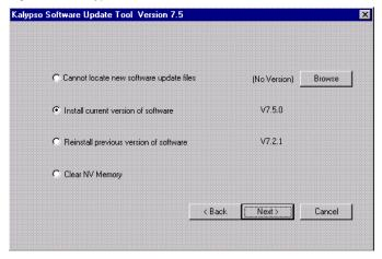
**3.** Select the **Install current version of software** option and touch the **Next>** button. The following screen appears (Figure 195).
