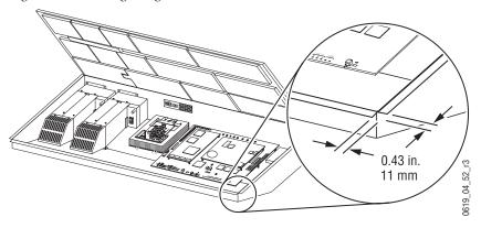
Figure 63. Main Panel Mounting Options (Front Left View)
