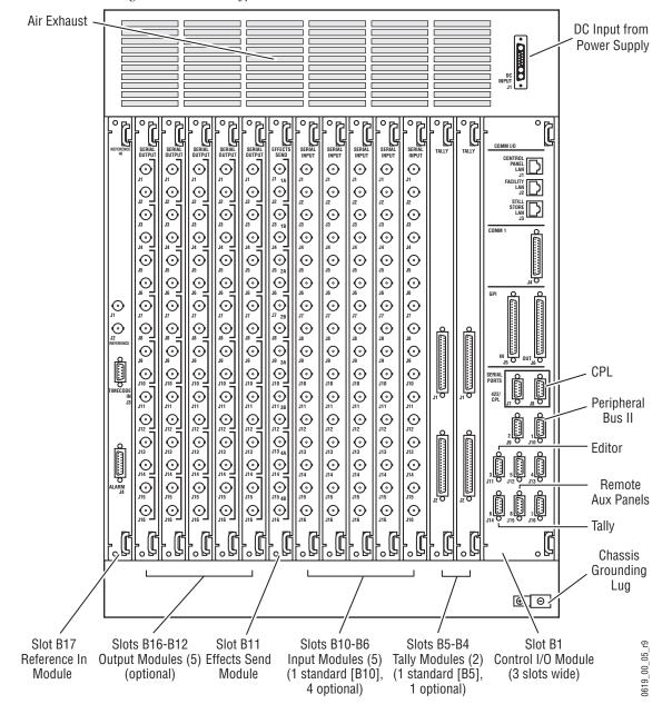
Figure 56. 4-M/E Kalypso Video Processor Frame, Rear View
