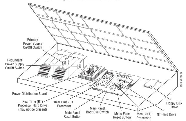
Figure 7. Early Model 4-M/E Main Panel Inside View
