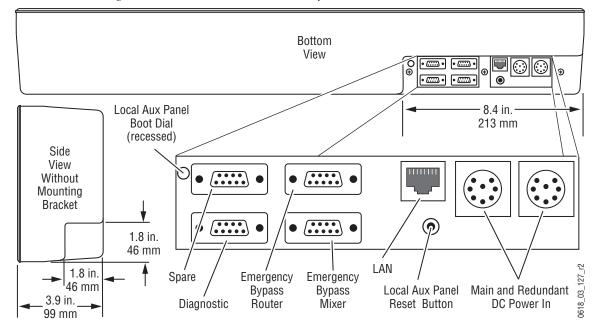
Figure 14. Local Aux Panel, Bottom View of Connectors
