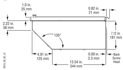
Figure 71. 2-M/E Main Panel Dimensions, Side View
