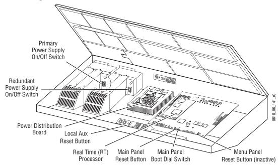
Figure 17. Late Model 2-M/E Main Panel, Inside View
