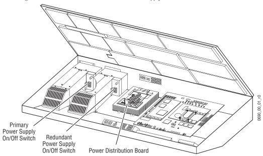
Figure 166. Power Distribution Board and Power Supply Switches
