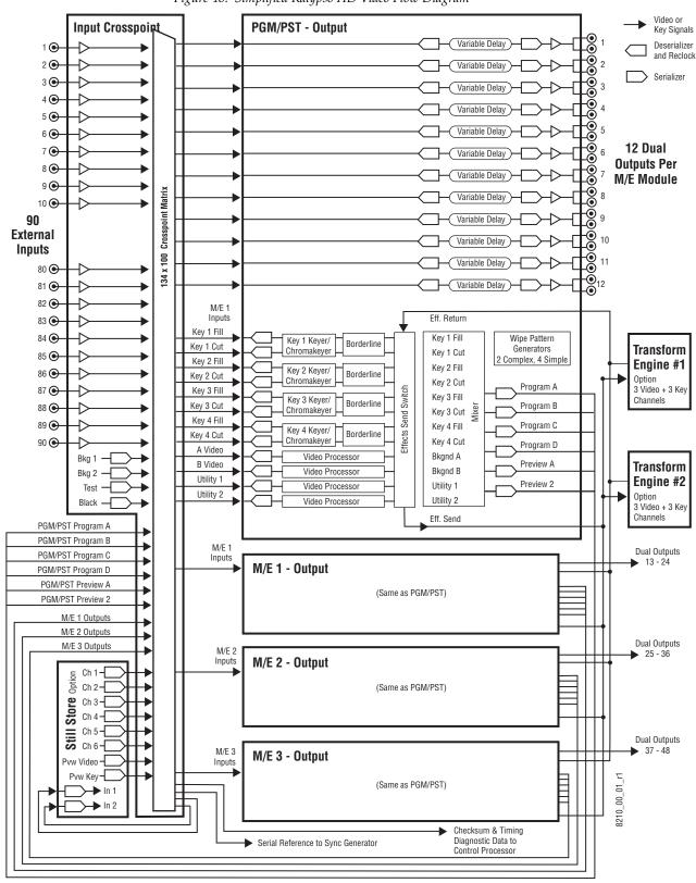
Figure 48. Simplified Kalypso HD Video Flow Diagram
