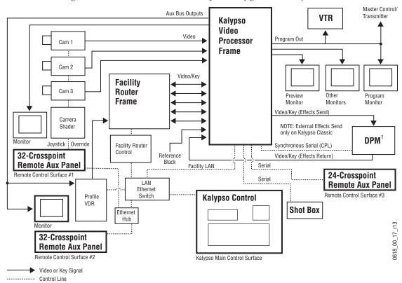
Figure 41. Basic Live Production Studio System Configuration Example
