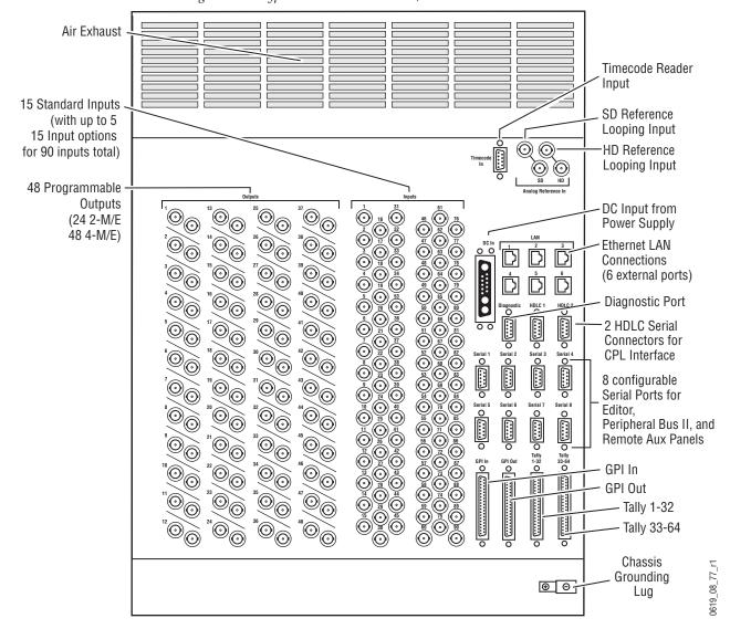
Figure 36. Kalypso Video Processor Frame, Rear View
