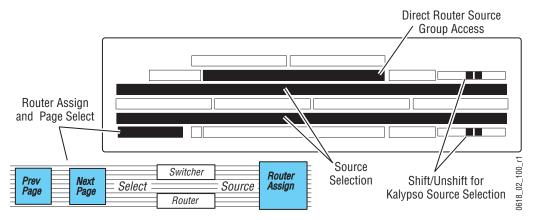
The **Router Assign** button on the Local Aux panel places that panel in Router Assign mode. All Aux Bus selection capabilities are disabled, replaced with router interface functions, and the button flashes to indicate this state. The Router light pipe also illuminates to show the current mode. Pressing **Router Assign** a second time exits Router Assign mode.
