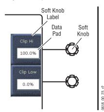
Knobs along the right side of the Menu panel can be used to dial in parameter values for functions displayed on the touch screen. When a knob is active, the touch screen displays the parameter name and its current value on a data pad (Figure 111). The parameter can be adjusted by turning the knob, or the data pad can be touched to bring up a numeric keypad.
