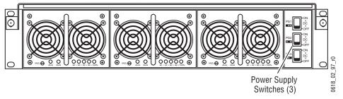
**2.** Set the power switch on the Video Processor Frame to On (Figure 118 for Kalypso Classic systems, Figure 119 on Kalypso HD/Duo systems).
