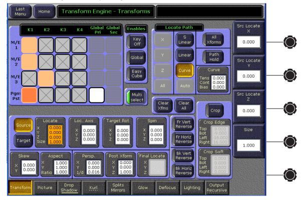
Figure 207. Transform Engine Menu, Multi-Select Enabled
