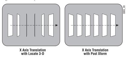
All post transform functions are made relative to the monitor screen frame of reference. For example, a positive X post transform always moves to the right side of the screen.
