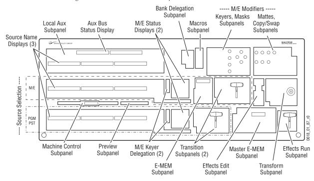
Figure 109. 2-M/E Main Panel and Subpanels
