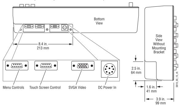
Figure 11. Original Menu Panel, Bottom View of Connectors
