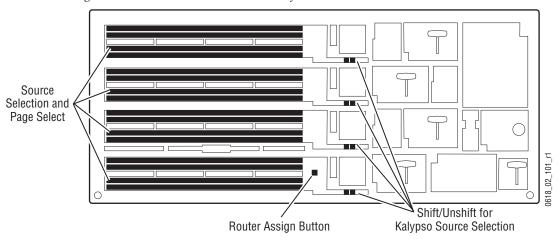
The **Router Assign** button on the Main panel is held down to place and keep the Main panel in Router Assign mode. When held down all normal panel operation is disabled, replaced with Router assign functions. Releasing the **Router Assign** button returns the Main panel to normal operation.
