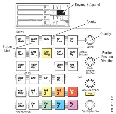
Figure 259. Keyers Subpanel, Borderline Controls
