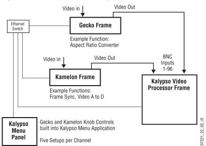
Figure 223. Newton Modular Control Diagram
