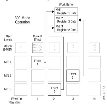
Figure 80. E-MEM 300 Mode Diagram
