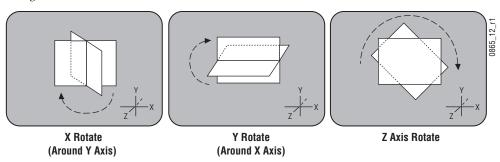
**Spin** — Supports multiple rotations about the reference axis in the X, Y, and Z directions. Spin supports fractional values, and is similar to Rotate when the move is less than  $\pm$ . one half revolution. Spin uses Euler math to calculate the move, which is not quite as precise as Quaternian, but permits multiple rotations. Spin applies transform values in Z, X, Y order, so editing effects in this axis order provides the best control of the effect.
