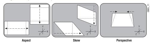
**Aspect** — Scaling the X or Y components of the picture. X axis changes affect horizontal size, Y axis changes affect vertical size (Figure 87). Z axis changes affect both X and Y dimensions, and is the same as Size.
