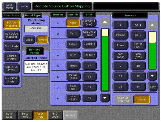
Figure 124. Remote Aux Panel Button Mapping Menu
