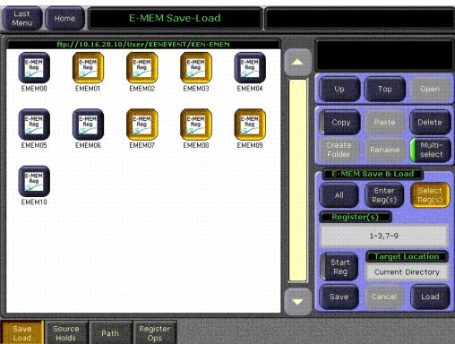
Figure 143. Multiselect Button Allows Selection of Multiple Files
