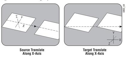
If the channel is controlled by a global channel, and the global channel itself has been rotated, an X axis translation will depend on whether the channel itself or the global channel is being manipulated, and whether source or target space is being used (Figure 91 and Figure 92). Note that the target translate of the channel is the same as a source translate of the global channel.
