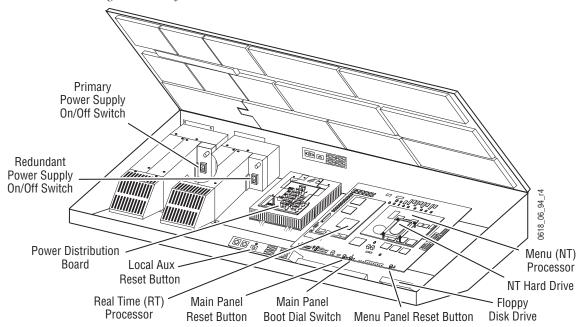
Figure 19. Early Model 2-M/E Main Panel, Inside View
