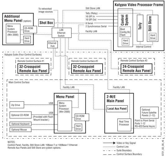
Early model Kalypso system control is shown in Figure 42 (4-M/E system) and Figure 43 (2-M/E system).
