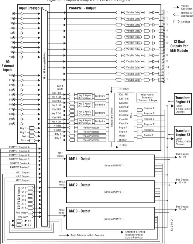
Figure 46. Simplified Kalypso HD Video Flow Diagram
