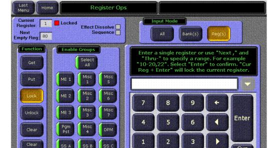
Figure 199. E-MEM Register Operations Menu, Lock Selected
