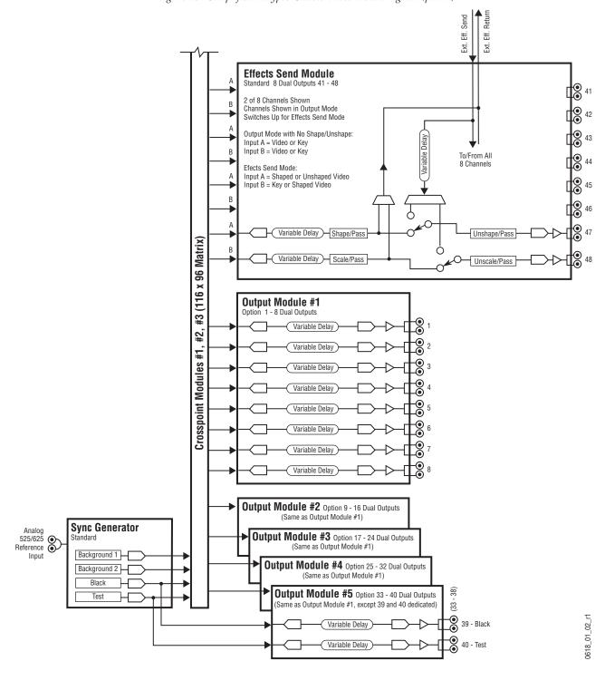
Figure 45. Simplified Kalypso Classic Video Flow Diagram (part 2)
