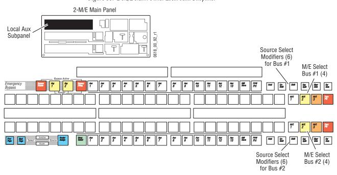
Figure 86. 2-M/E Main Panel Local Aux Subpanel
