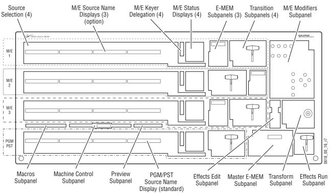
Figure 47. 4-M/E Main Panel and Subpanels
