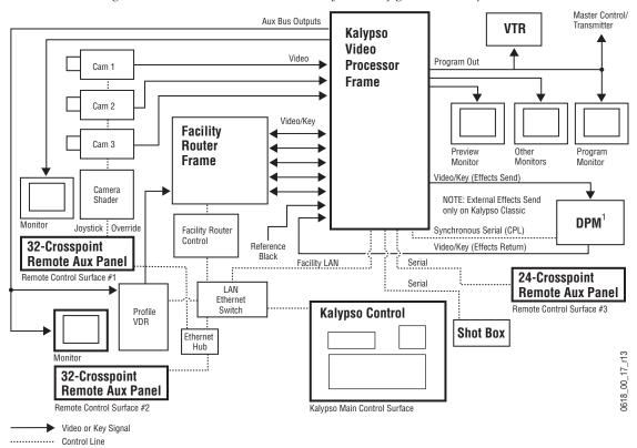
Figure 39. Basic Live Production Studio System Configuration Example
