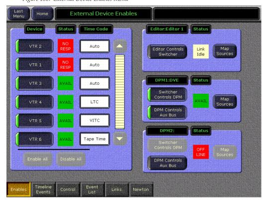
Figure 158. External Device Enables Menu
