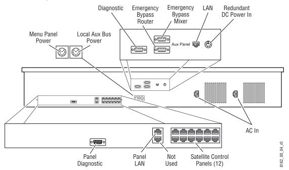
Figure 16. Late Model 2-M/E Main Panel, Rear View
