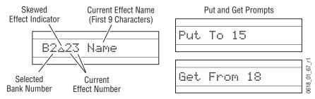
If there is more than one current effect register (different E-MEM levels were independently recalled from different registers, also called a *skewed effect*) a triangle symbol is displayed between the current bank number and the current register number. The locations of the contributing registers can be determined by turning on one enable at a time.
