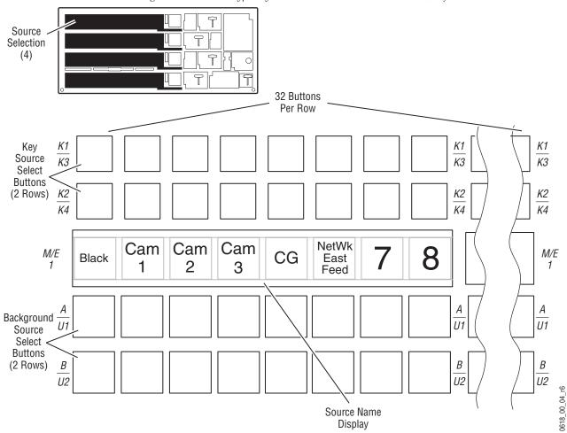
Figure 48. 4-M/E Kalypso System Source Selectors on Main Panel, Left Side
