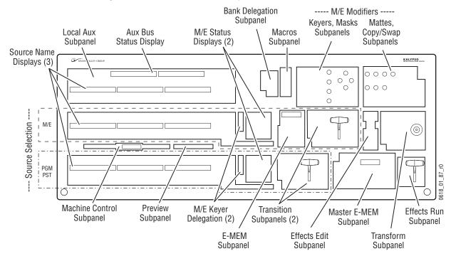
Figure 81. 2-M/E Main Panel and Subpanels
