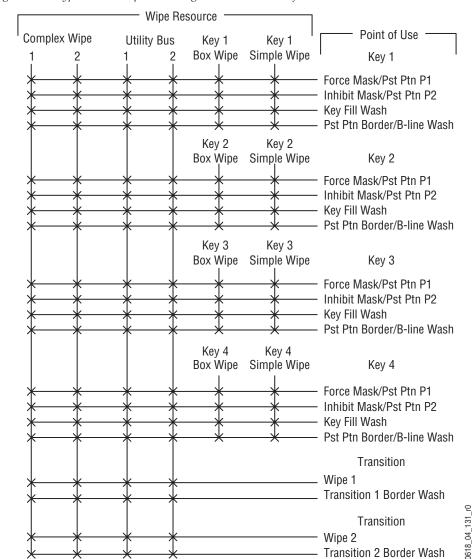
Figure 270. Typical M/E Wipe Switching Matrix and Point of Use
