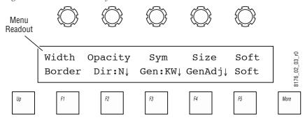
The readout display labels the functions of the soft knobs above and the soft buttons below. Seven characters of the display are used for each knob and button.
