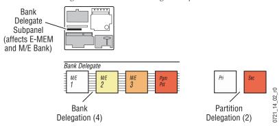
When M/E 1, M/E 2, or M/E 3 is selected, that Kalypso system M/E is controlled by the 1-M/E panel, and the E-MEM subpanel operates the same as an individual M/E E-MEM on a 2 or 4-M/E Kalypso Main panel.
