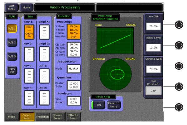
Figure 245. Video Processing Menu – Luminance Proc Amp Controls
