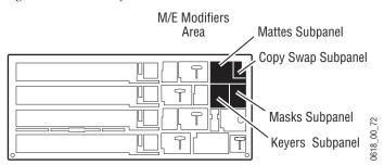
Delegation determines which M/E and keyer, or matte is being controlled at any given time by the M/E Modifiers controls. Delegation is available on the individual subpanels, via the M/E Keyer delegation buttons, and can be configured to occur automatically. See the *Kalypso User Manual* for more information on Delegation.
