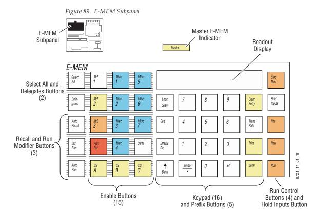
The E-MEM subpanel operates as either an individual M/E E-MEM subpanel or as a Master E-MEM subpanel, depending on delegation.
