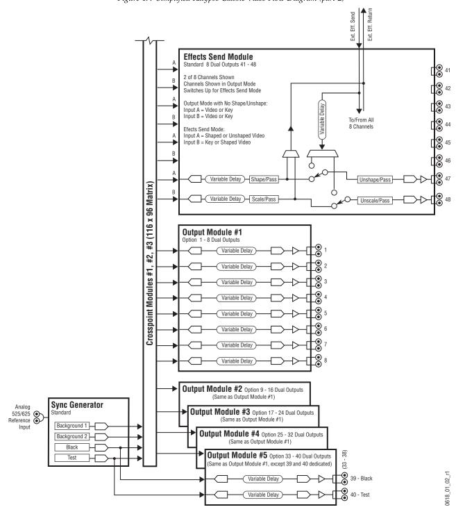
Figure 47. Simplified Kalypso Classic Video Flow Diagram (part 2)
