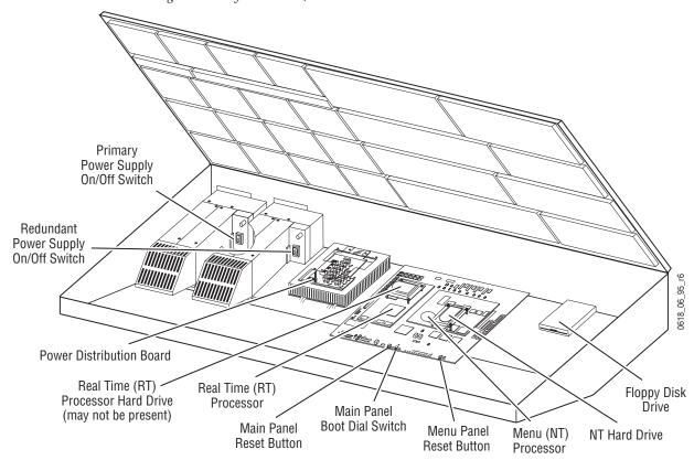
Figure 7. Early Model 4-M/E Main Panel Inside View
