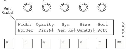
The readout display labels the functions of the soft knobs above and the soft buttons below. Seven characters of the display are used for each knob and button.
