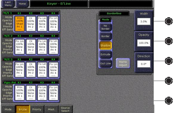
The 4 x 4 grid of data pads on the left are used to delegate one of the 16 keyers. The Borderline controls displayed for the delegated keyer on the right side match the button and knob controls on the Main panel.
