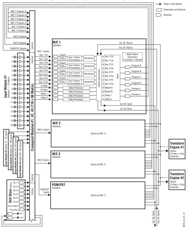
Figure 46. Simplified Kalypso Classic Video Flow Diagram (part 1)
