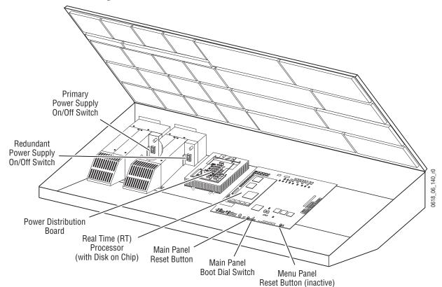
Figure 5. Late Model 4-M/E Main Panel Inside View
