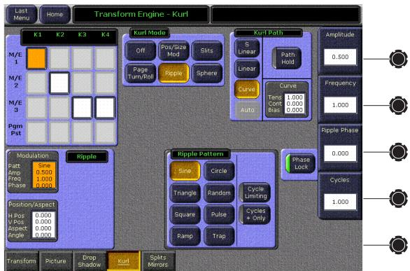
Figure 251. Kurl Menu, Ripple Modulation
