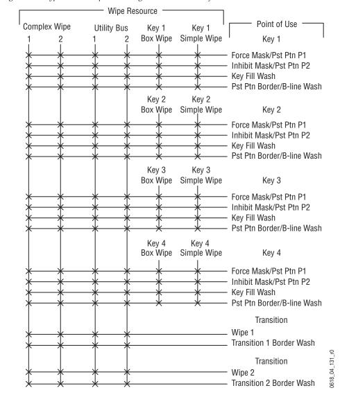
Figure 287. Typical M/E Wipe Switching Matrix and Point of Use
