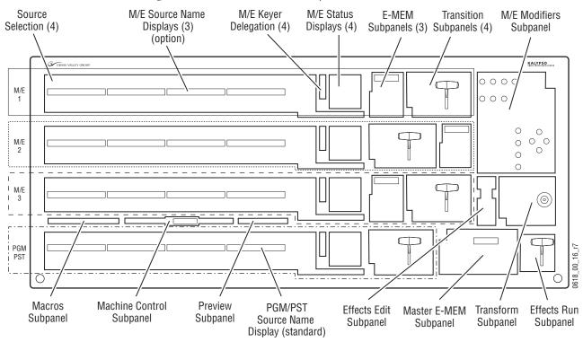
Figure 49. 4-M/E Main Panel and Subpanels
