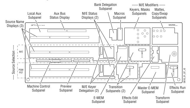
Figure 83. 2-M/E Main Panel and Subpanels
