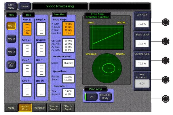
Figure 262. Video Processing Menu – Luminance Proc Amp Controls
