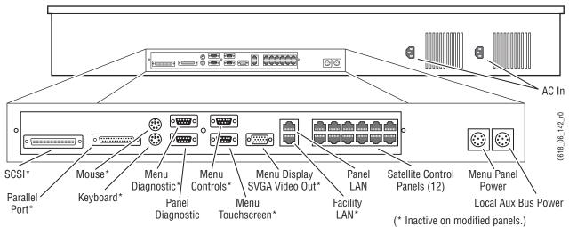
Figure 6. Early Model 4-M/E Main Panel, Rear View
