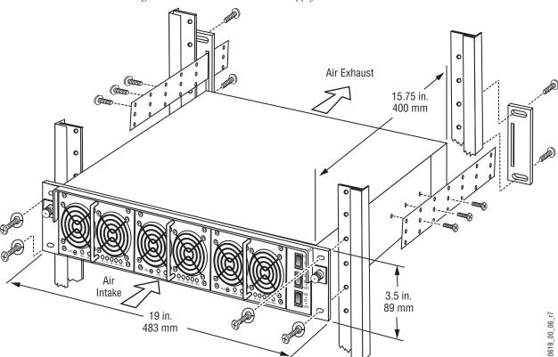
Figure 45. Video Processor Power Supply Installation
