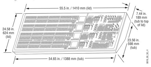
Figure 53. 4-M/E Rear Main Panel Dimensions
