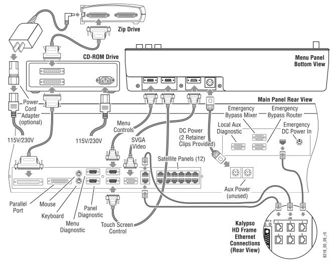
Figure 103. Early Model 2-M/E Control Surface Cabling
