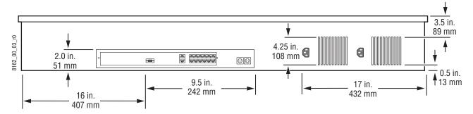
Figure 54. 4-M/E Main Panel Dimensions, Side View
