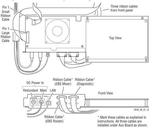
Figure 153. Local Aux Processor Interface Board Cabling
