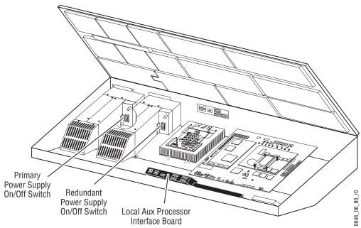
Figure 152. Local Aux Processor Interface Board Location
