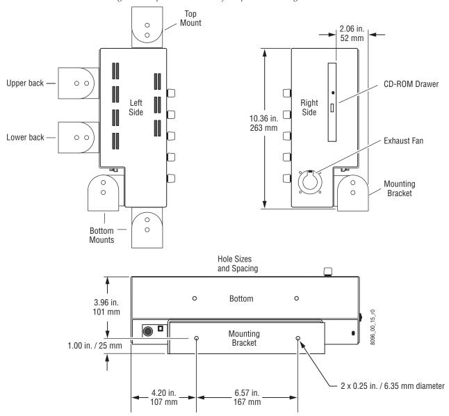
Figure 81. Optional Placement of Adaptable Mounting Bracket
