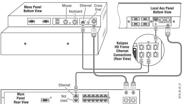
Figure 33. Kalypso 4-M/E Bench Test Ethernet Cabling
