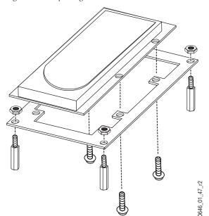
Figure 150. Replacing Board Mounted Hard Drives
