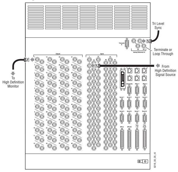
Figure 40. Bench Test Video Connections
