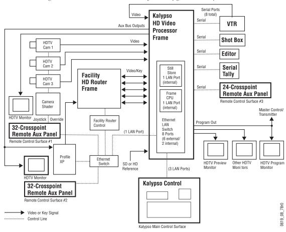
Figure 29. Basic Live Production Studio System Configuration Example
