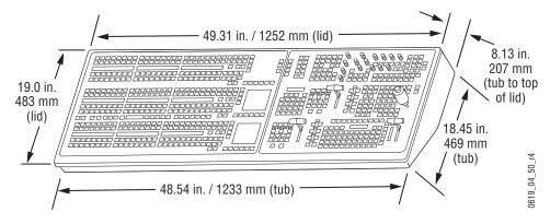
Figure 56. 2-M/E Rear Panel Dimensions
