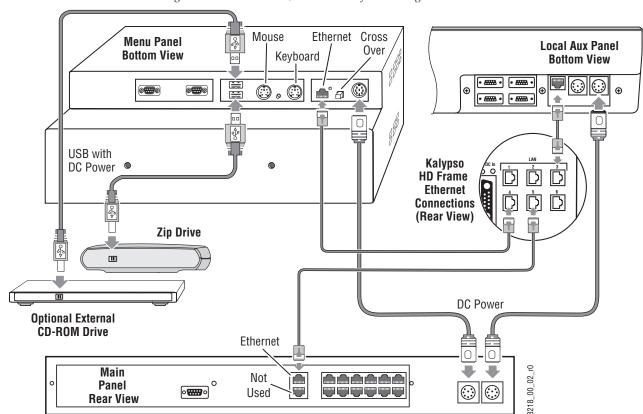
Figure 93. Standard 4-M/E Control Surface Cabling
