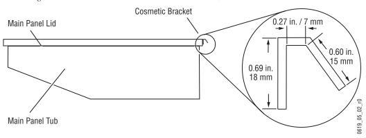
If you choose to use the cosmetic bracket and your Main panel installation has a console support structure similar to that shown in Figure 51, it will be necessary to cut notches in the support members at the left and right rear corners of the console cutout (see the notch dimensions in Figure 51). This enables the Main panel lid to clear the support structure upon opening.
