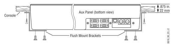
Figure 91. Local Aux Panel Console Flush Mount
