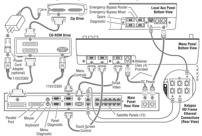
Figure 102. Early Model 4-M/E Control Surface Cabling
