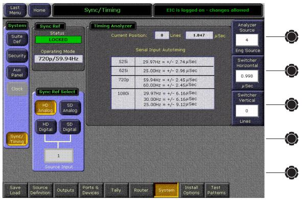
Figure 98. Sync/Timing Menu, HD System
