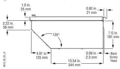
Figure 57. 2-M/E Main Panel Dimensions, Side View
