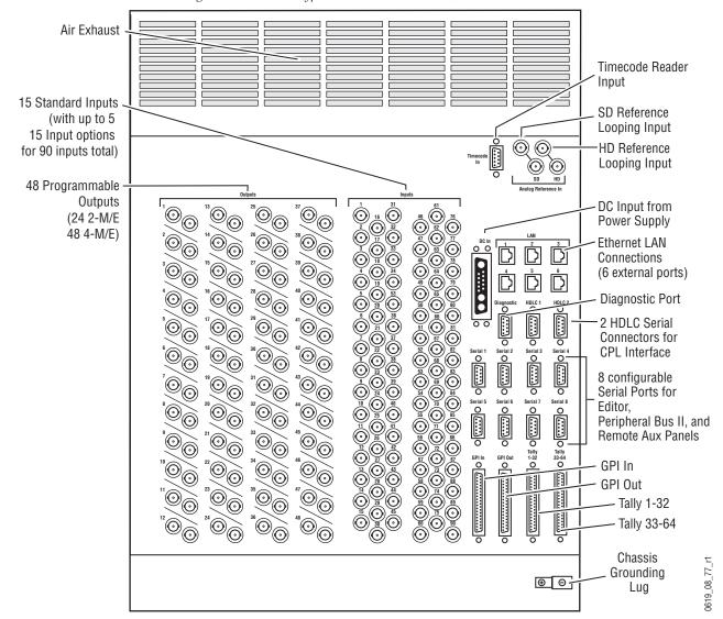
Figure 44. 4-M/E Kalypso Video Processor Frame, Rear View
