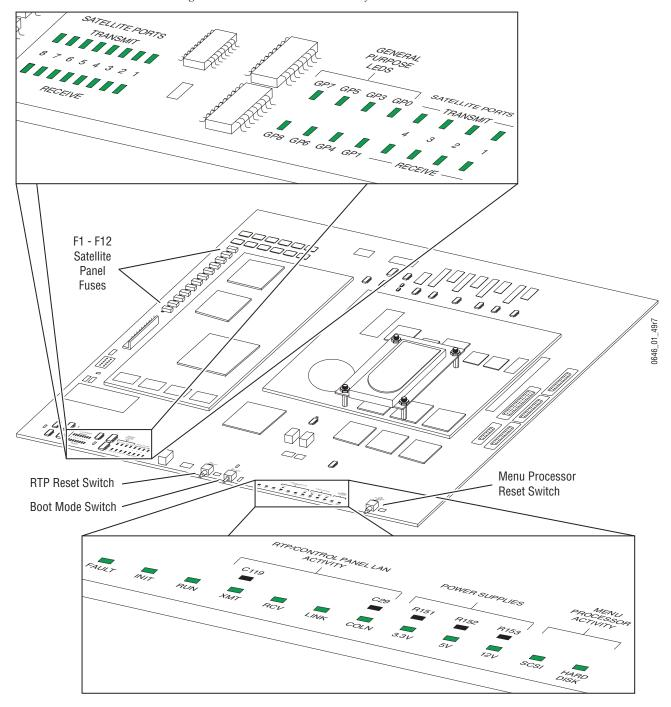
Figure 157. Real Time Processor Interface Board Status Indicators
