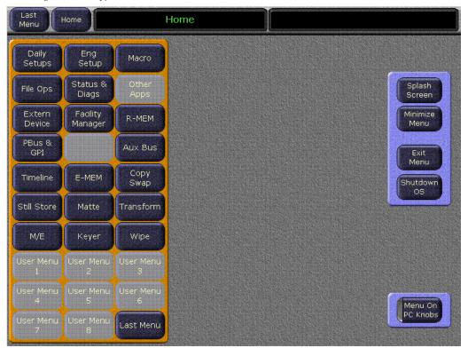
17. Touch the **Status & Diags** button to go to the Versions menu (Figure 37). The software reported for each system component should be the latest version, and all the versions should be the same (if the Still Store option is not installed its version will be blank). This confirms the correct Kalypso software is loaded on all system components.
