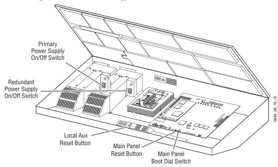
Figure 173. Late Model 2-M/E Kalypso Main Panel Reset Switches
