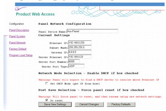
Figure 114. Typical Kalypso System Default IP Address Settings
