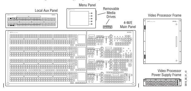
Figure 1. 4-M/E Kalypso System Components
