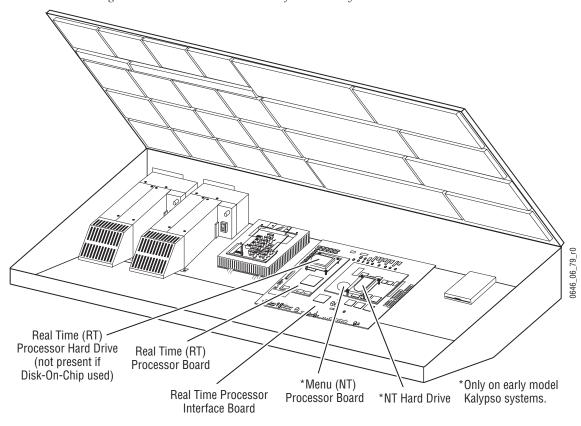
Figure 151. Real Time Processor Interface Assembly
