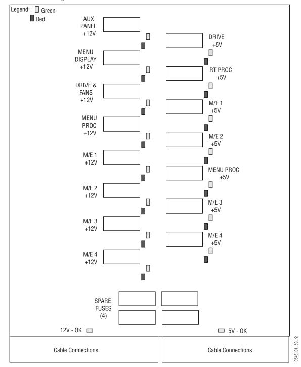
Figure 160. Main Panel Power Distribution Board Fuse and Status Indicators
