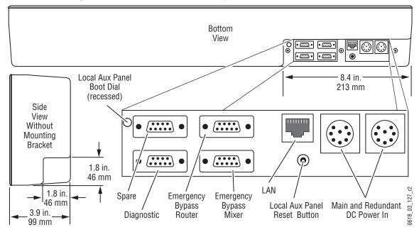
Figure 10. Local Aux Panel, Bottom View of Connectors
