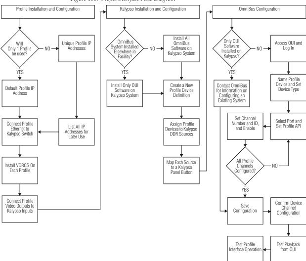
Figure 193. Profile Interface Flow Diagram
