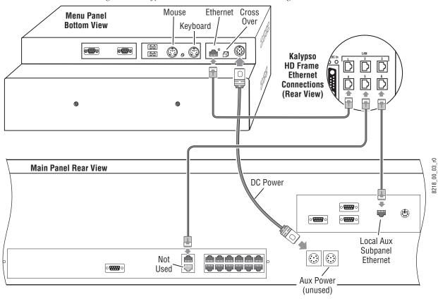
Figure 34. Kalypso 2-M/E Bench Test Ethernet Cabling
