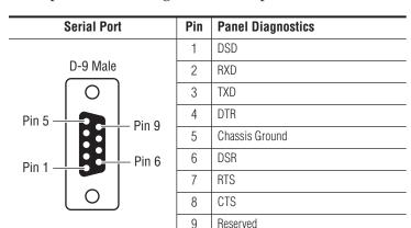
Main panel Panel Diagnostic serial port are shown below.
