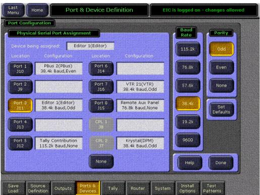
Figure 181. Ports & Devices – Port Configuration Menu
