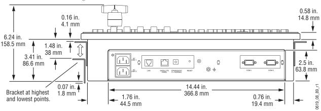
Figure 60. 1-M/E Rear Panel Dimensions
