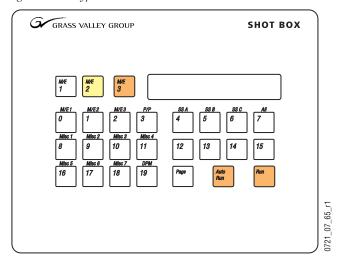
The Shot Box can be powered from the Main panel through the cables provided. If located more than 3 m (10 ft) from the Main panel, an optional Satellite Panel extension kit is available that includes a brick type power supply.
