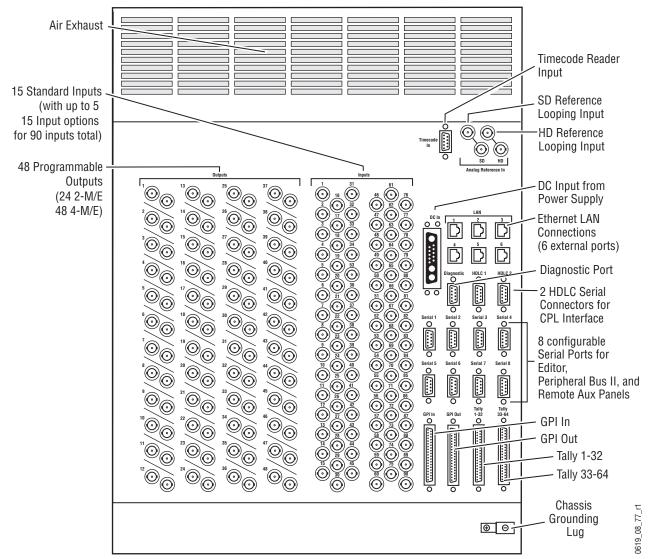
Figure 26. Kalypso Video Processor Frame, Rear View
