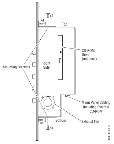
Figure 84. Attaching Flush Mount Bezel to Menu Panel
