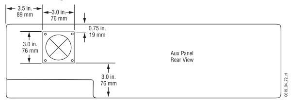
Figure 92. Local Aux Panel Fan Position
