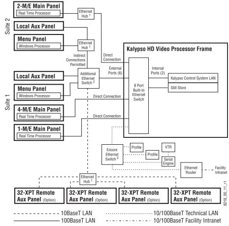
Figure 96. Example Topography Requiring Additional Ethernet Switches
