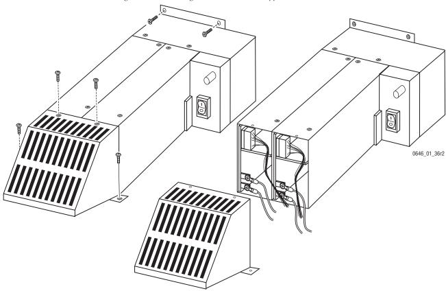
Figure 156. Removing Main Panel Power Supplies
