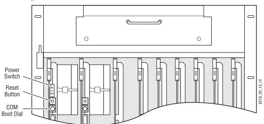
Figure 110. Control Module Reset Button and COM Boot Dial Switch
