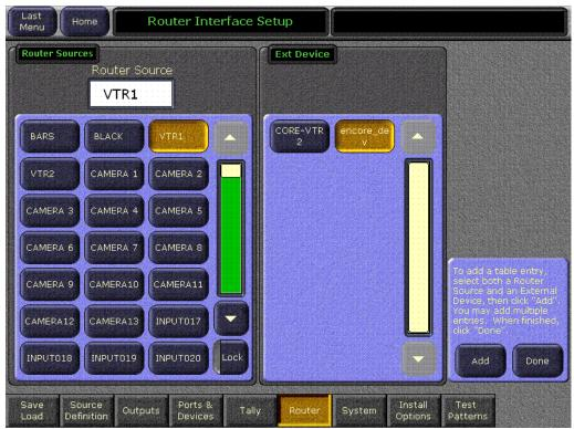
Figure 205. Router Source and External Device Mapping Menu
