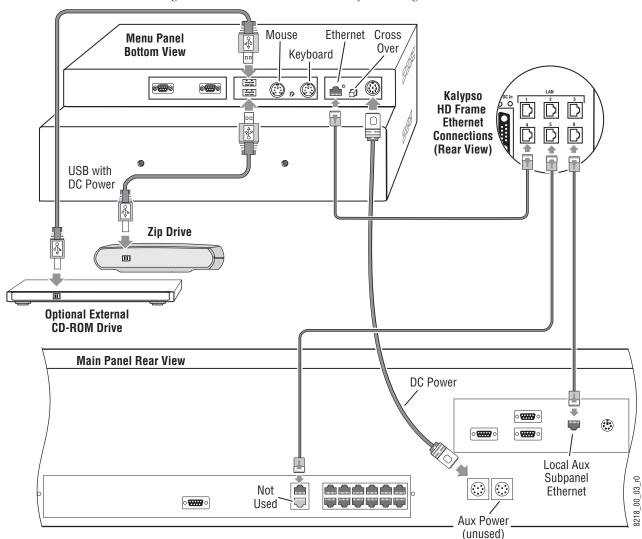
Figure 94. Standard 2-M/E Control Surface Cabling
