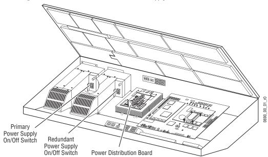
Figure 148. Power Distribution Board and Power Supply Switches
