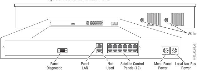
Figure 4. 4-M/E Main Panel, Rear View
