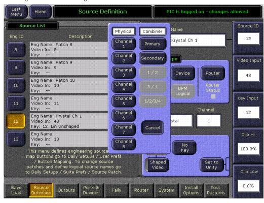
Figure 189. Channel Assignment Selection Pane
