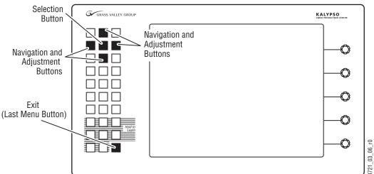
Figure 144. Original Menu Panel Screen Adjustment Control Buttons
