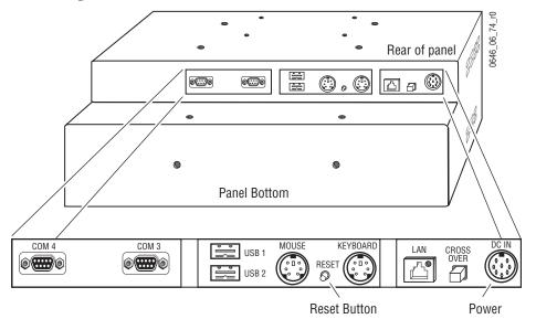
Figure 174. Enhanced Menu Panel Reset Button Location
