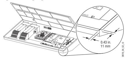
Figure 49. Main Panel Mounting Options (Front Left View)
