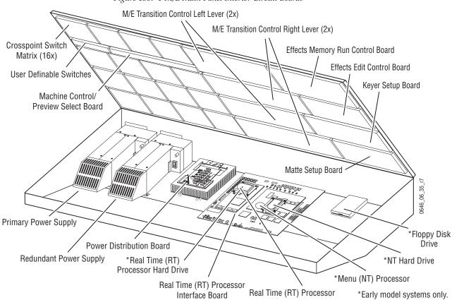
Figure 158. 4-M/E Main Panel Interior Circuit Boards
