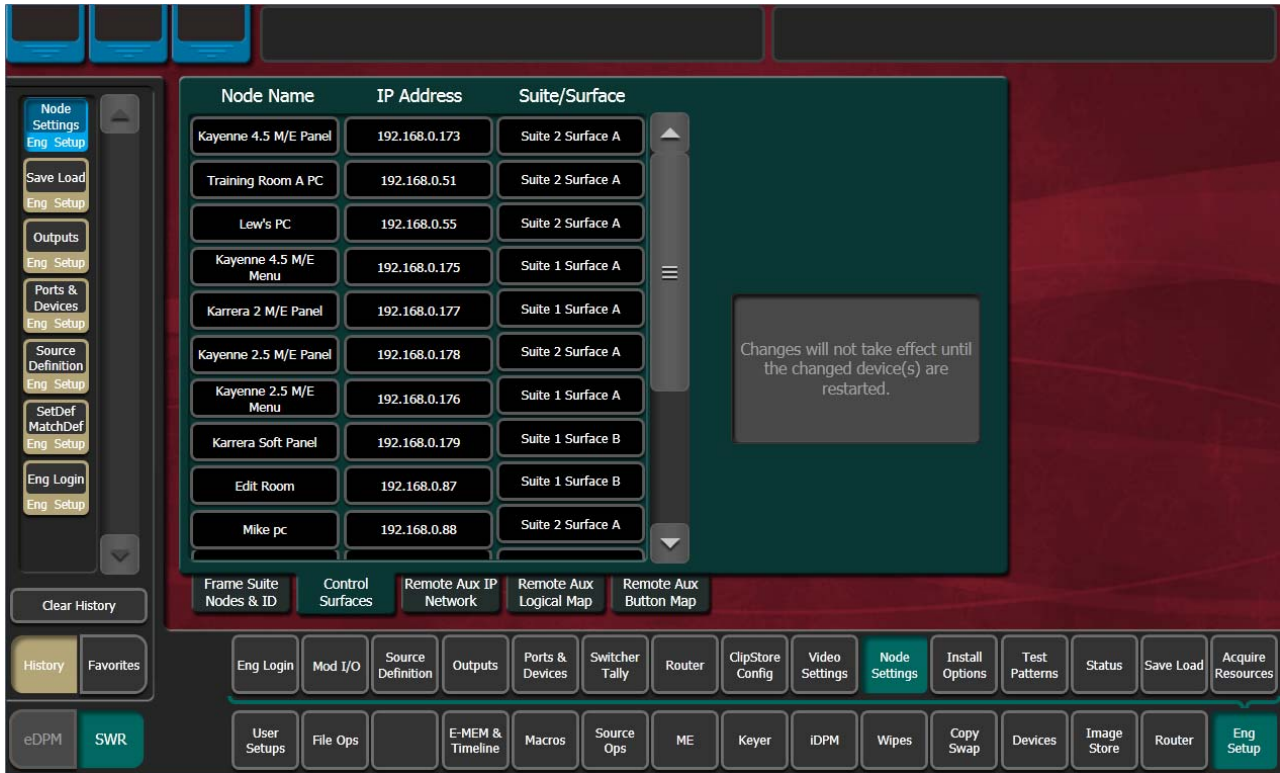
Figure 123. Control Surface Menu with Suite 2 PC and Panel
