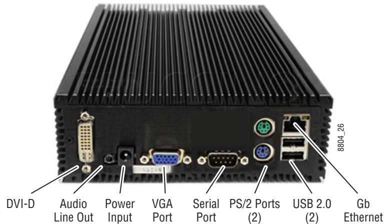
Figure 21. Fanless PC Rear Connectors
