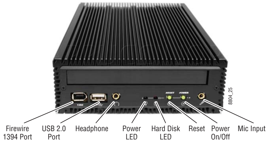
Figure 20. Fanless PC Front Connectors
