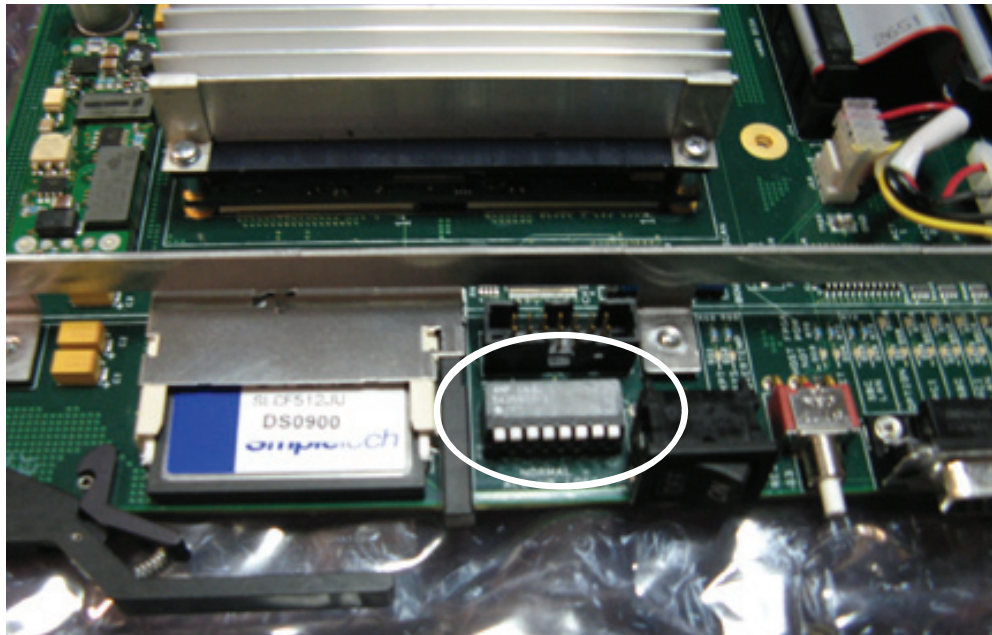
Figure 106. Kayak Control Processor Board - S2 Boot Mode Dipswitch Location
