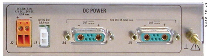
Figure 34. KDD-PSU DC Power Connectors
