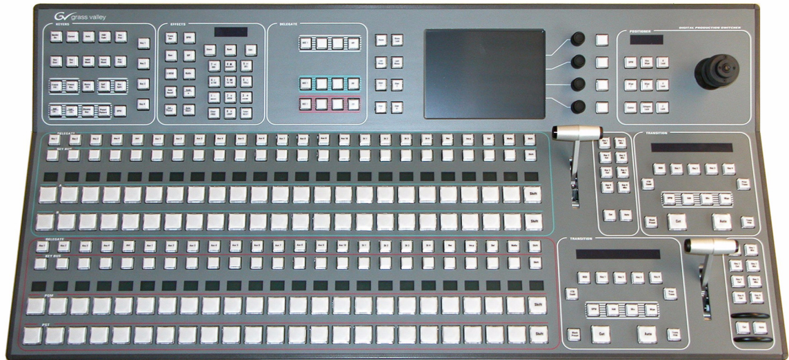
Figure 3. Kayak HD 150C, 200C, and 200 Control Panel
