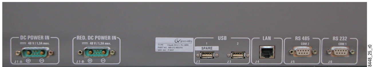
Figure 31. Kayak HD Control Panel Rear Connectors
