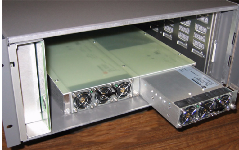
Figure 23. KHD-PSU Internal Redundant Power Supply Option
