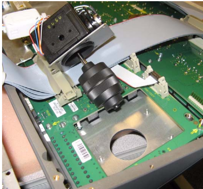
Figure 131. Kayak Control Panel Joystick—Removing the Joystick
