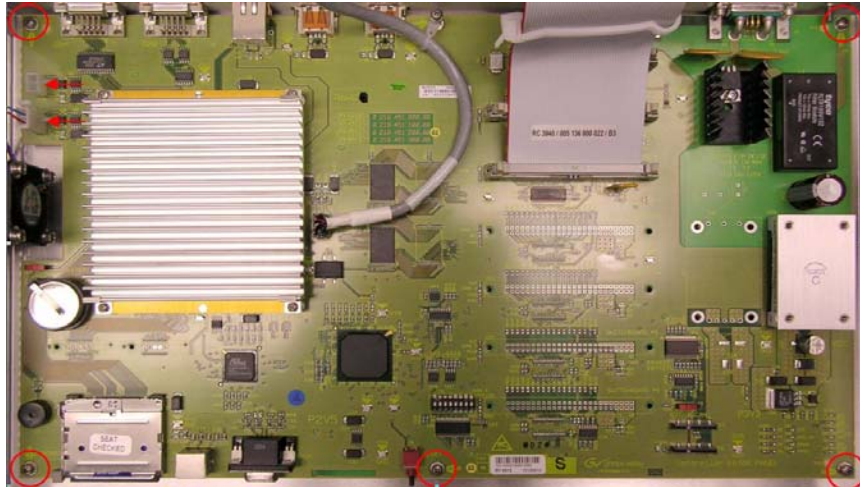
Figure 122. Kayak Control Board—Tub Screw Removal
