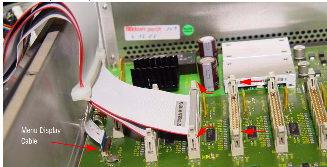
Figure 116. Kayak Control Panel—Ribbon Cable Removal
