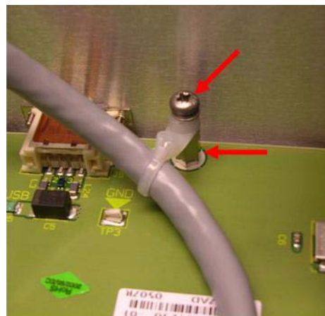
Figure 123. Kayak Control Board—Screw and Hex Stand-off Removal
