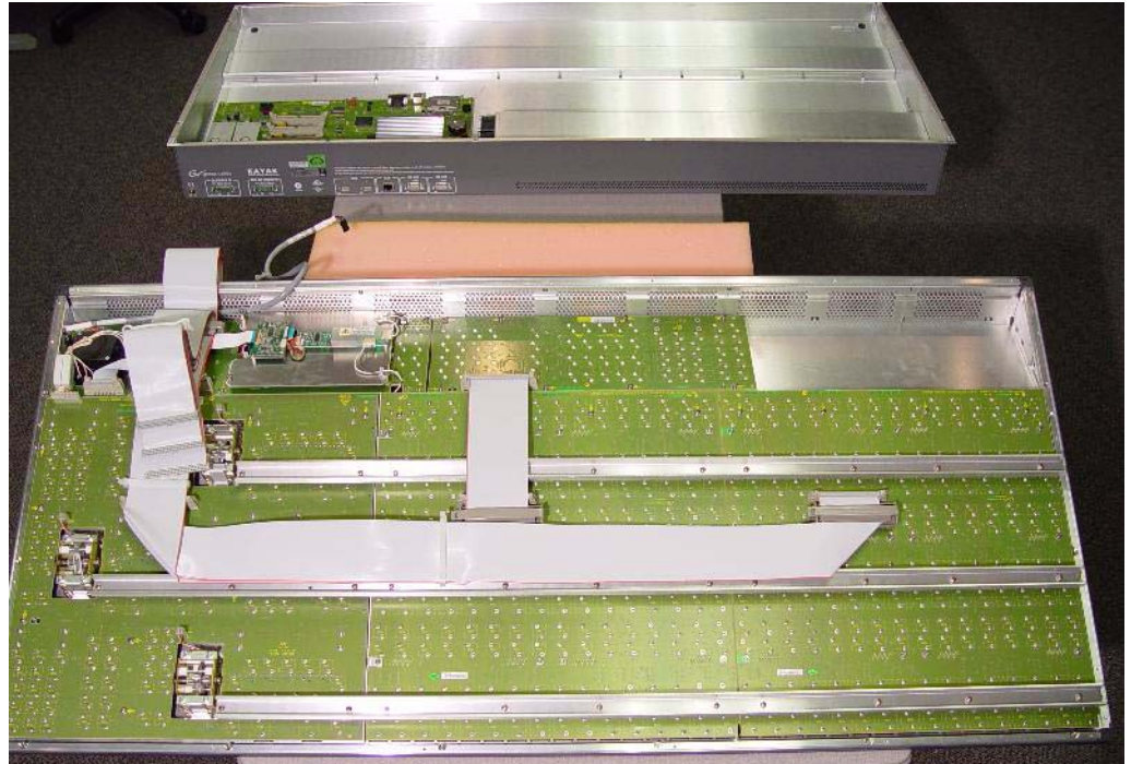
Figure 118. Kayak Control Panel—Separated Enclosure
