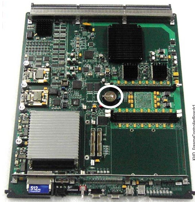
Figure 110. Kayak HD Frame Controller Board with Battery in center of board
