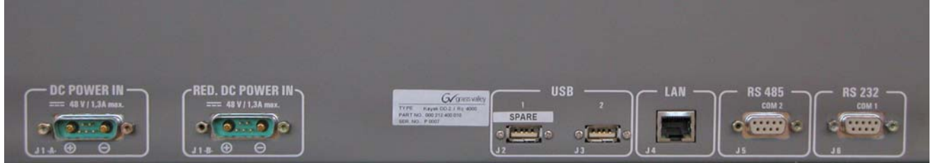
Figure 13 Control Panel Connectors
