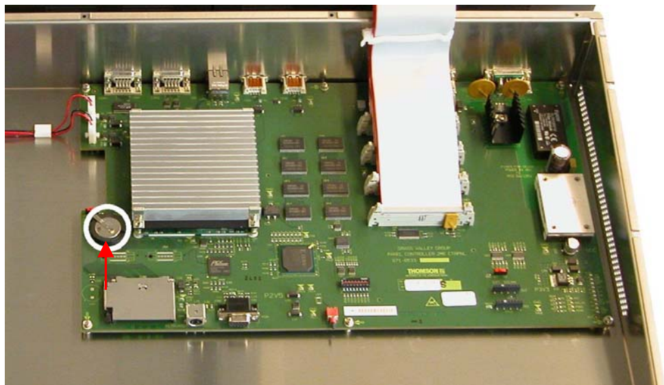
Figure 36 Battery on the Board of the Control Panel
