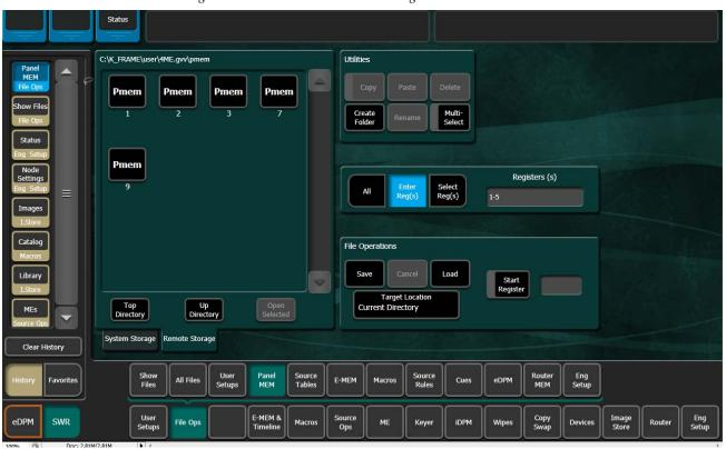
Figure 37. Panel MEM Menu—Load Registers
