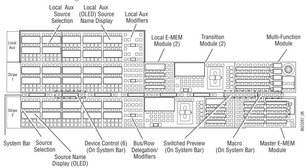
Figure 106. 2-ME Control Panel and Modules
