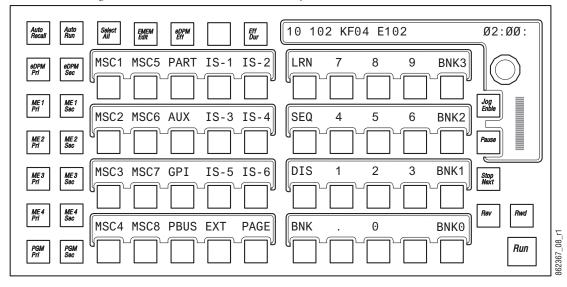
Figure 113. Master E-MEM Module Example
