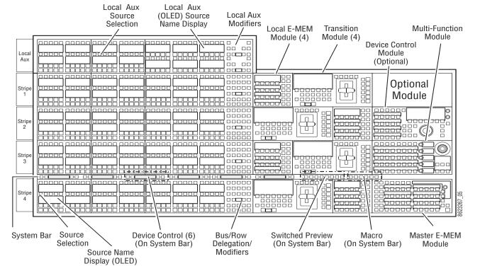
Figure 105. 4-ME Control Panel and Modules
