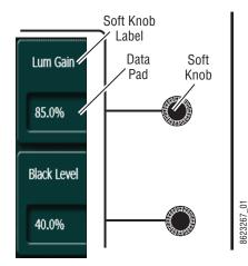
Knobs along the right side of the Menu Panel can be used to dial in parameter values for functions displayed on the touch screen. When a knob is active, the touch screen displays the parameter name and its current value on a data pad. The parameter can be adjusted by turning the knob, or the data pad can be touched to bring up a numeric keypad.
