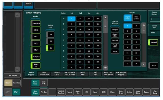
Figure 12. Button Mapping Menu, Logical Sources
