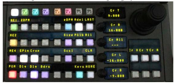
Figure 191. Multi-Function Module—2D-DPM Edge Pinning, Crop
