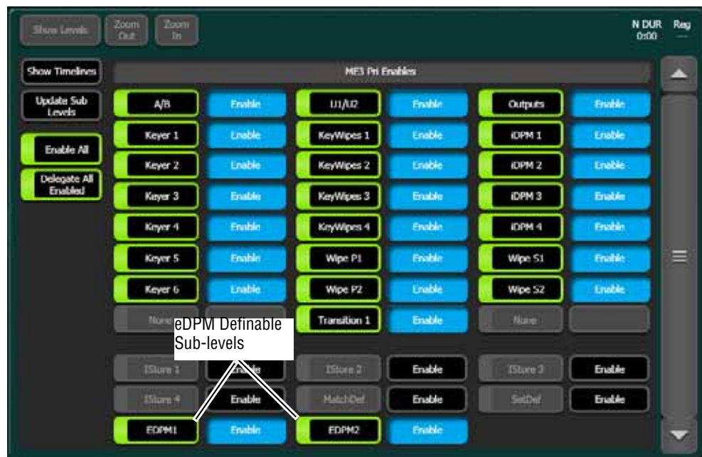
Figure 72. eDPM Sub-levels in the E-MEM Master Timeline
