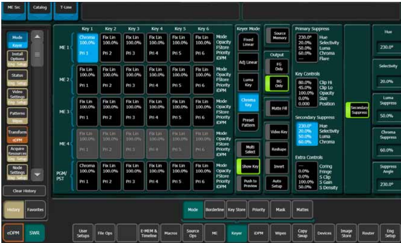
Figure 50. Sec Suppress Controls—Six Keyer System
