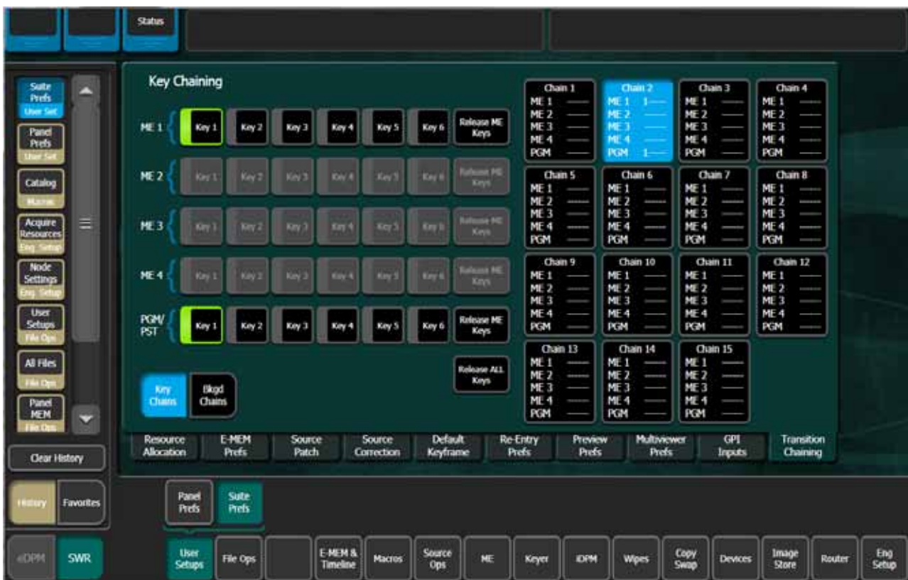
Figure 189. Multiple ME Key Chaining—Six Keyer System
