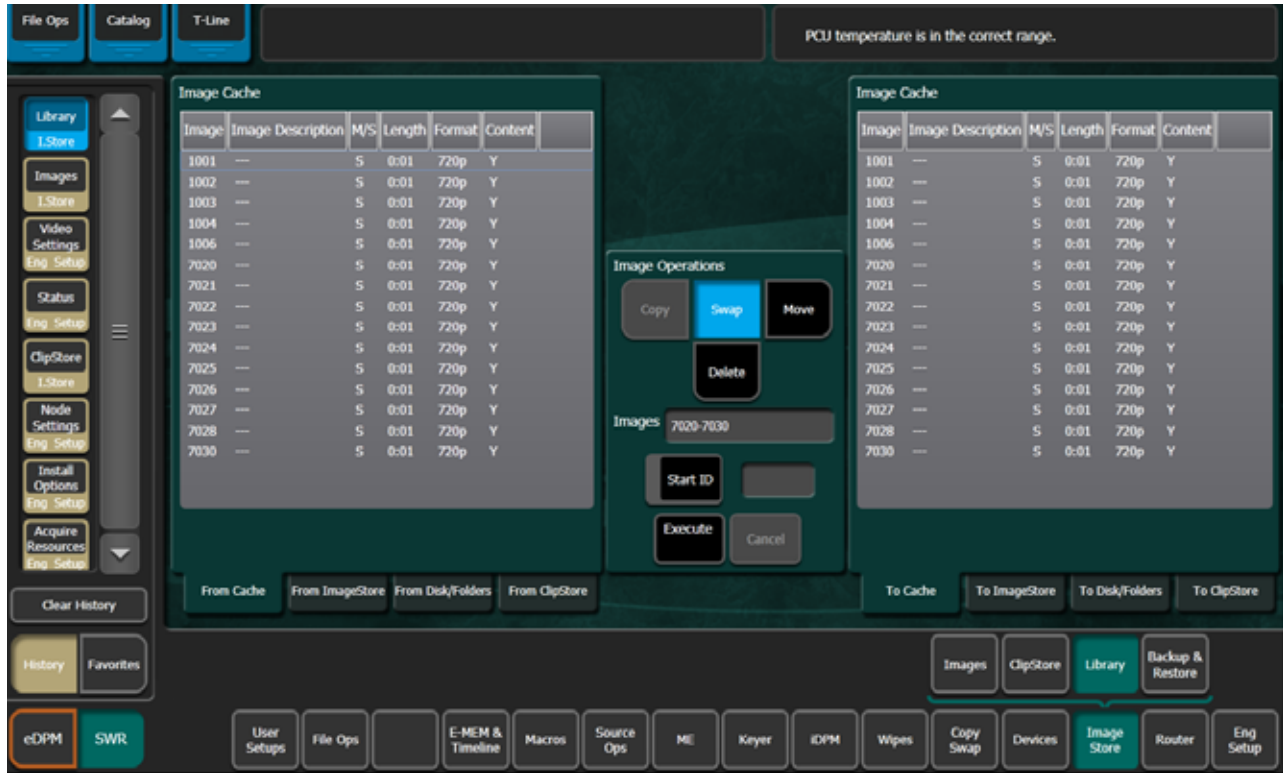
Figure 254. From Cache/To Cache, Move Operation
