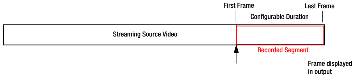
Figure 251. Image Store Delay Line Record Mode Definition
