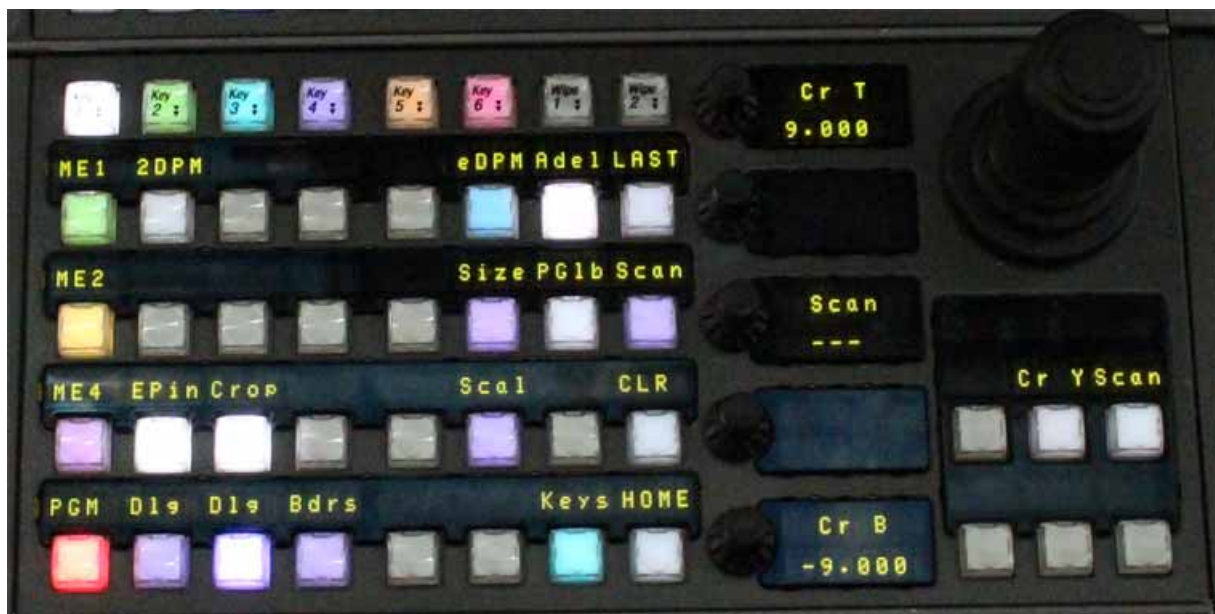
Figure 208. Multi-Function Module—2D-DPM Edge Pinning, Pan/Scan
