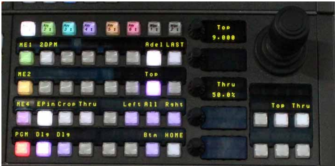
Figure 207. Multi-Function Module—2D-DPM Edge Pinning, EPin
