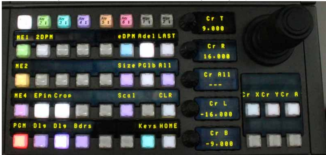
Figure 206. Multi-Function Module—2D-DPM Edge Pinning, Crop
