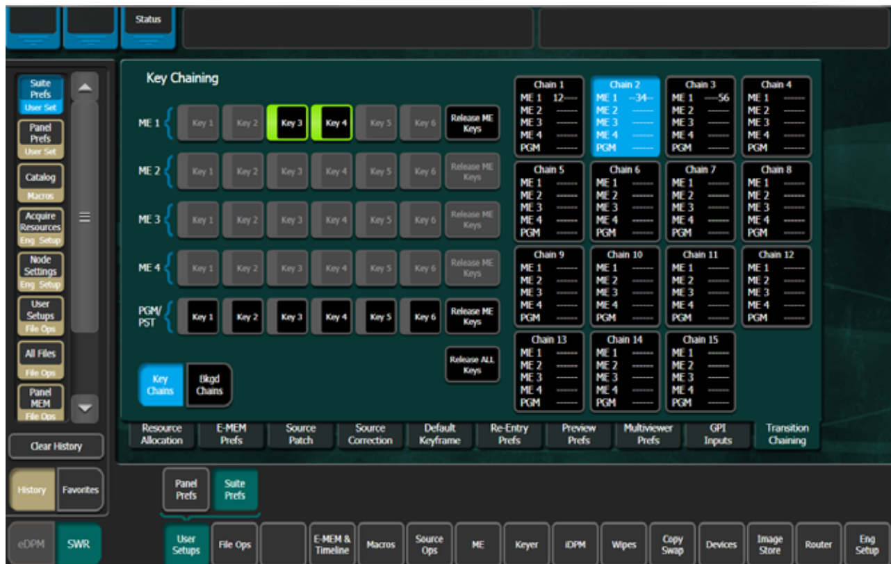
Figure 188. Single ME Key Chaining—Six Keyer System
