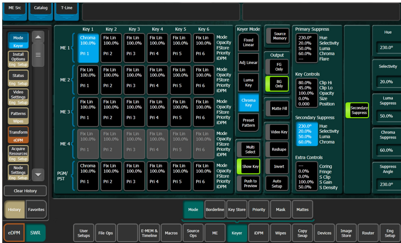
Figure 50. Sec Suppress Controls—Six Keyer System
