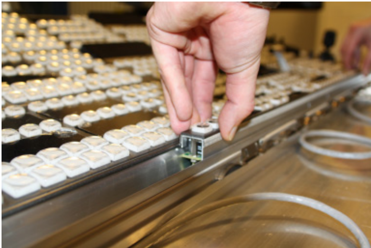
Aligning the System Bar for Replacement
