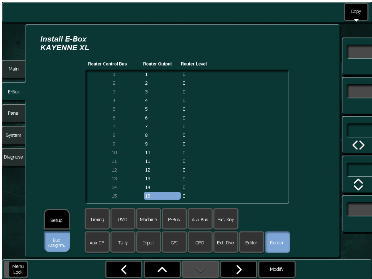
Figure 238. Install E-Box Router Bus Assignment
