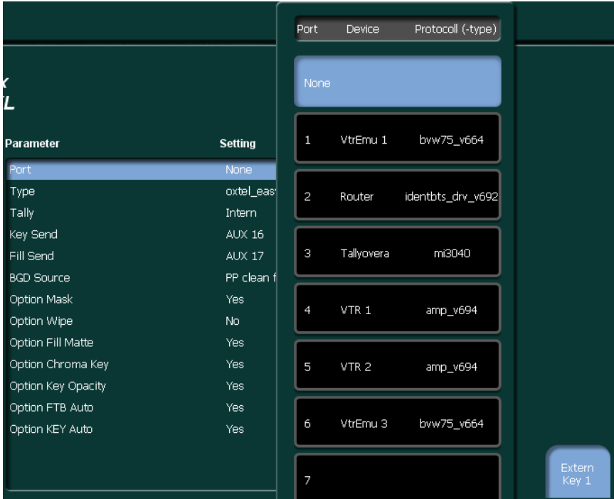
Figure 259. Install E-Box Extern Key Port
