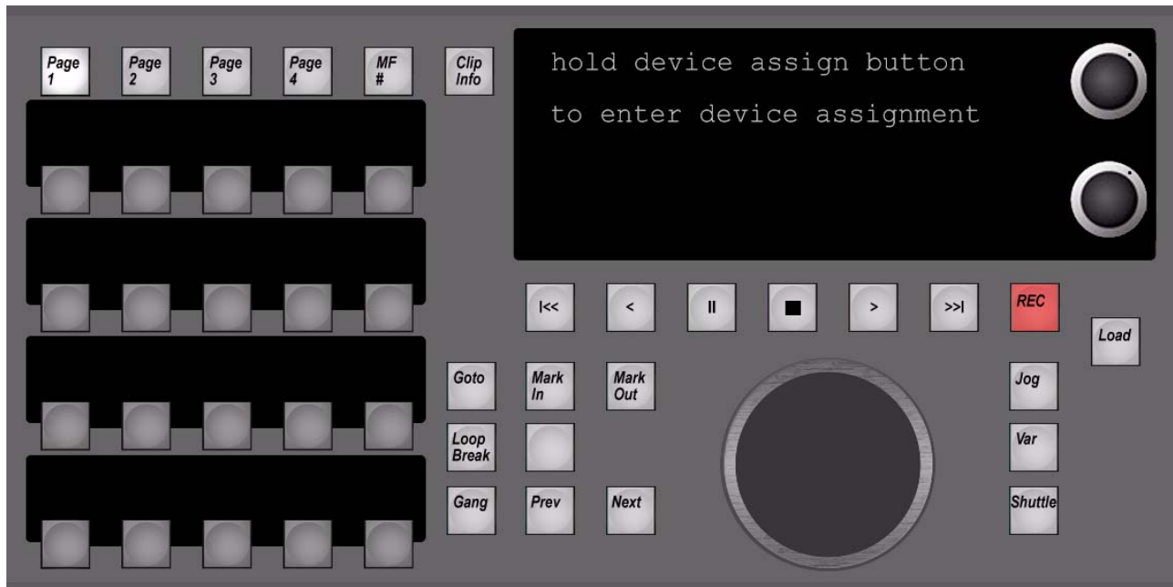
Figure 92. Machine Control Module
