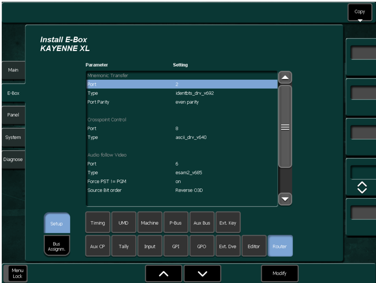
Figure 237. Install E-Box Router
