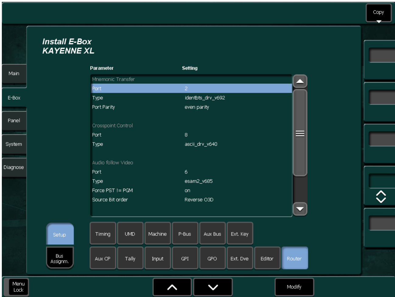
Figure 241. Install E-Box Router
