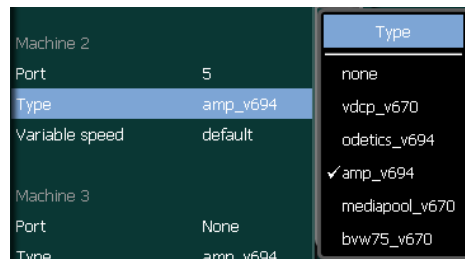
Figure 253. Install E-Box Machine Control Set Type
