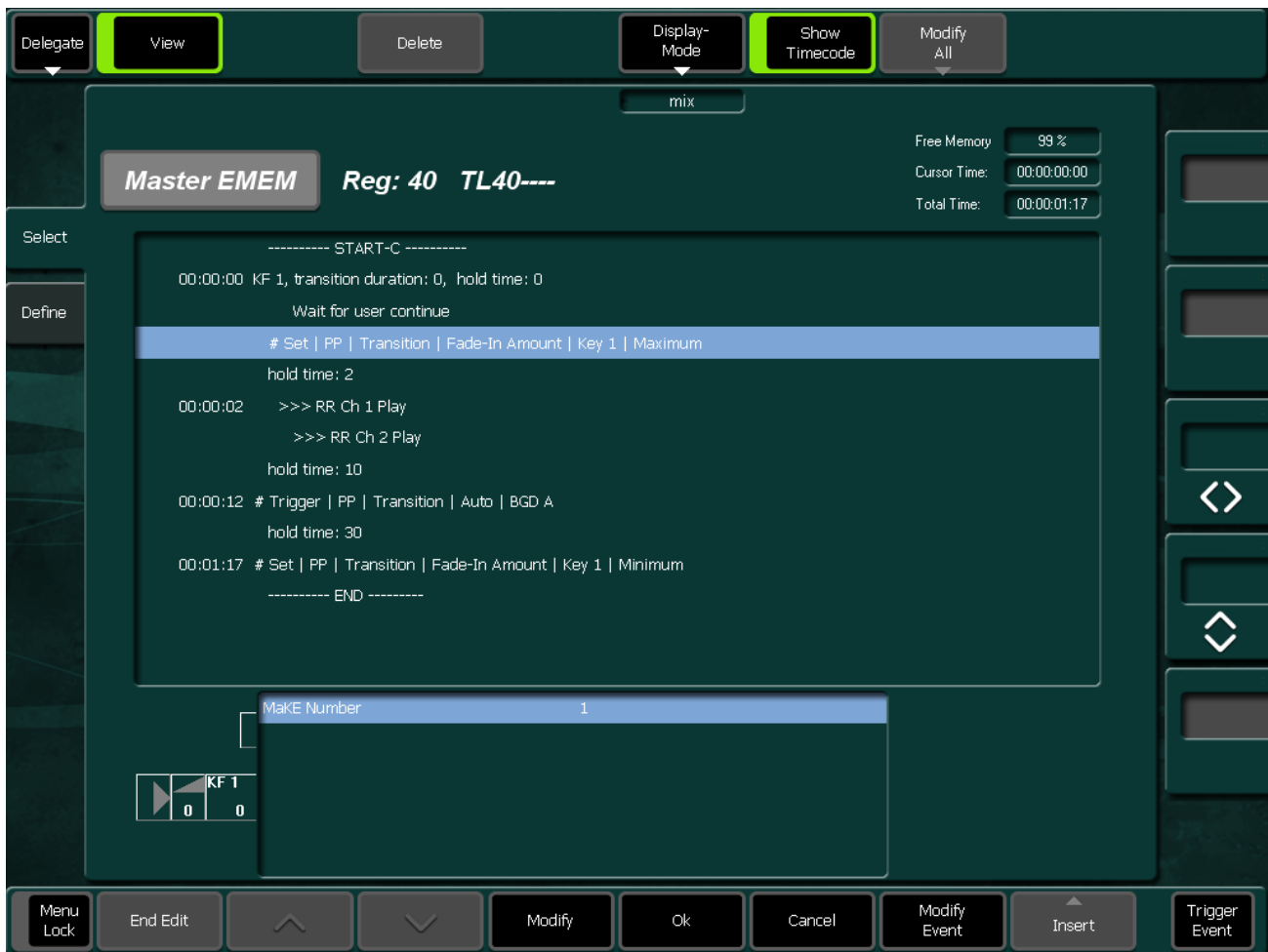
Figure 471. EMEM Edit Insert Trigger Macro
