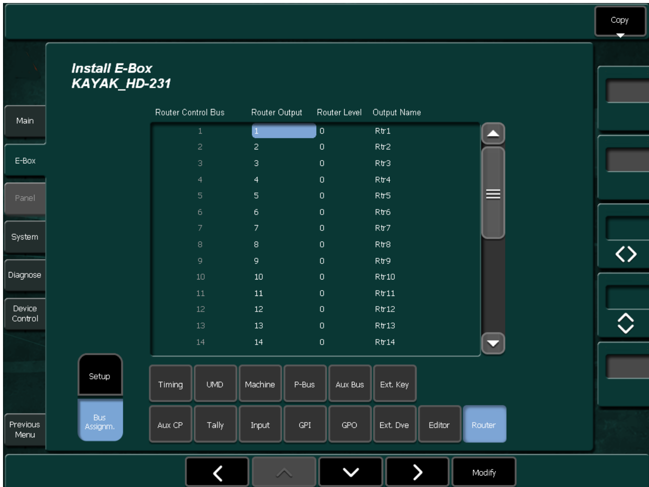
Figure 242. Install E-Box Router Bus Assignment
