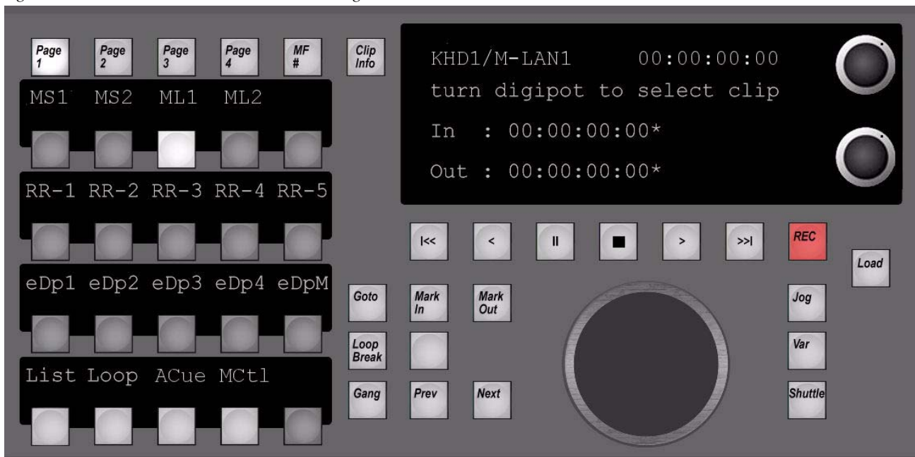
Figure 106. Machine Control - External VTR Delegation
