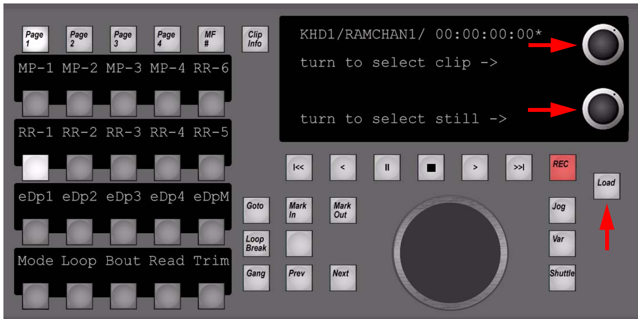
Figure 107. Machine Control - RamRecorder Delegation
