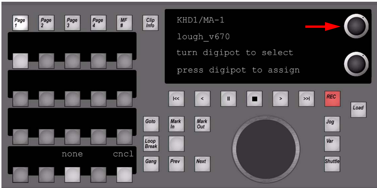
Figure 104. Machine Control - Digipots
