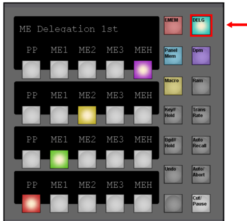
Figure 93. Selecting Half M/EMachine Control
