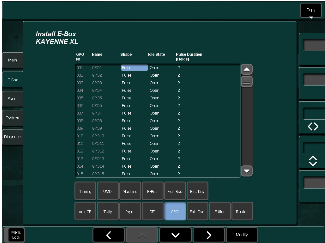
Figure 224. Install E-Box GPO
