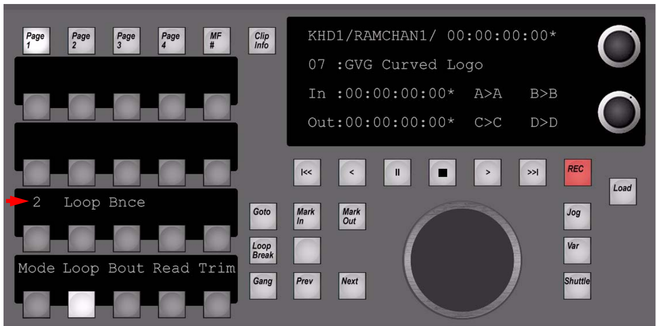
Figure 113. Machine Control - Loop
