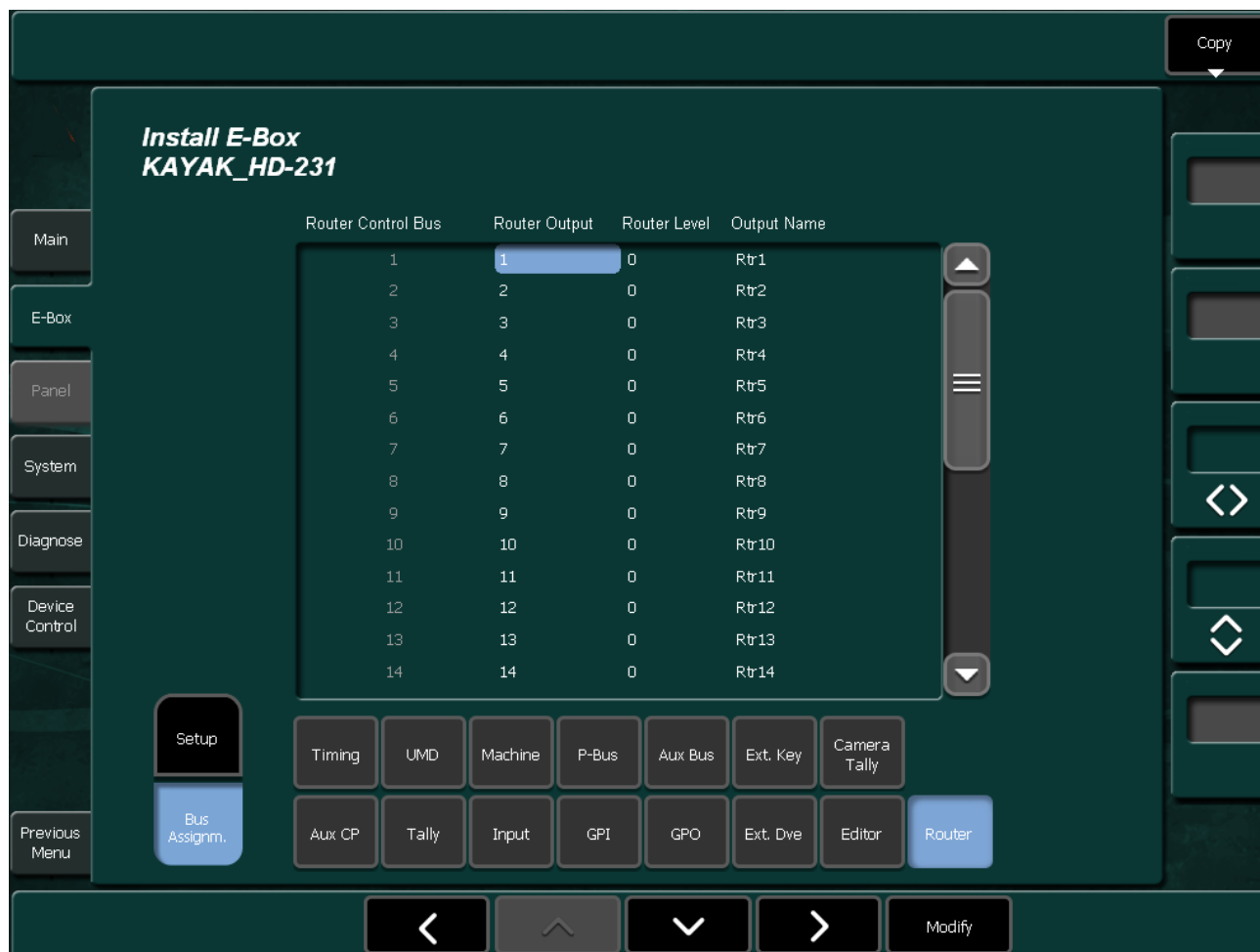
Figure 246. Install E-Box Router Bus Assignment
