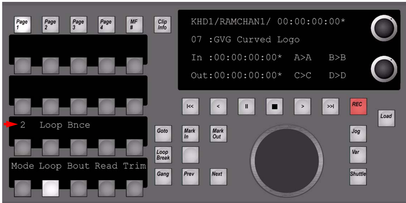
Figure 113. Machine Control - Loop
