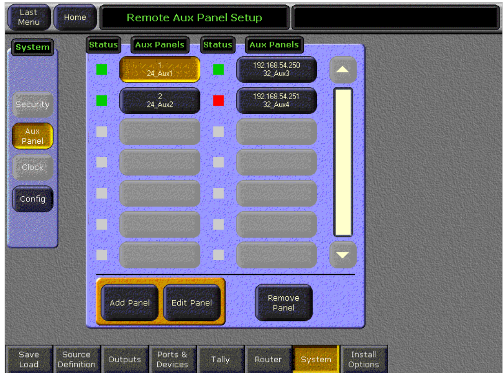
Figure 79. Eng Setup – System – Aux Panels Assigned
