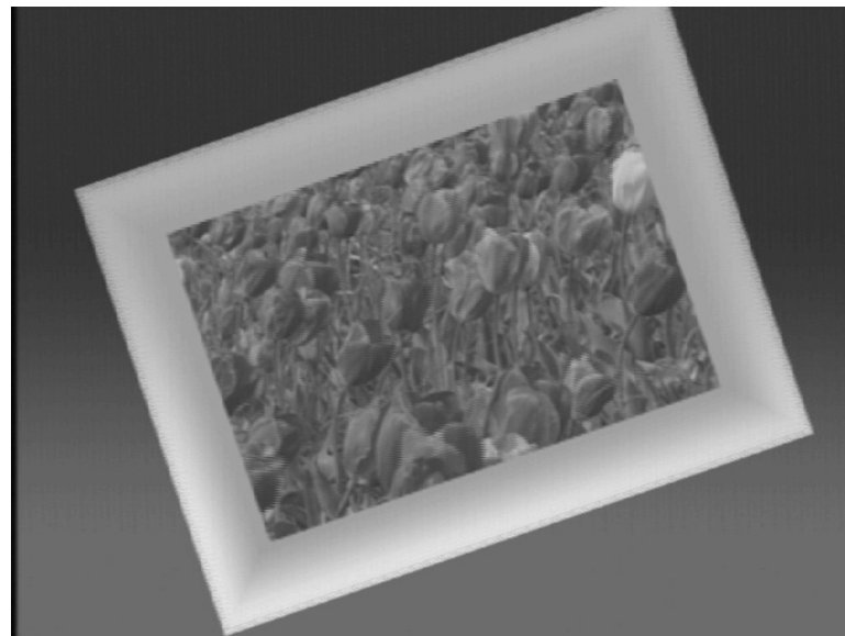
Figure 29. Incorrect Key With White Halo
