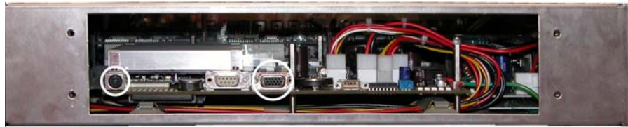
Figure 37 PS2 and VGA sockets on the KayakDD-1 Frame
