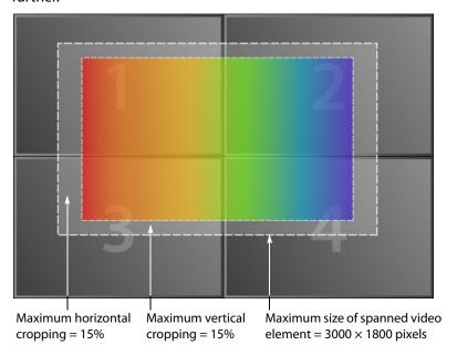
**Note:** Even if a spanned video monitor does not exceed the recommended maximum size, the problem could occur if it is set to follow AFD/WSS with a custom cropping of (15, 15, 15, 15).
