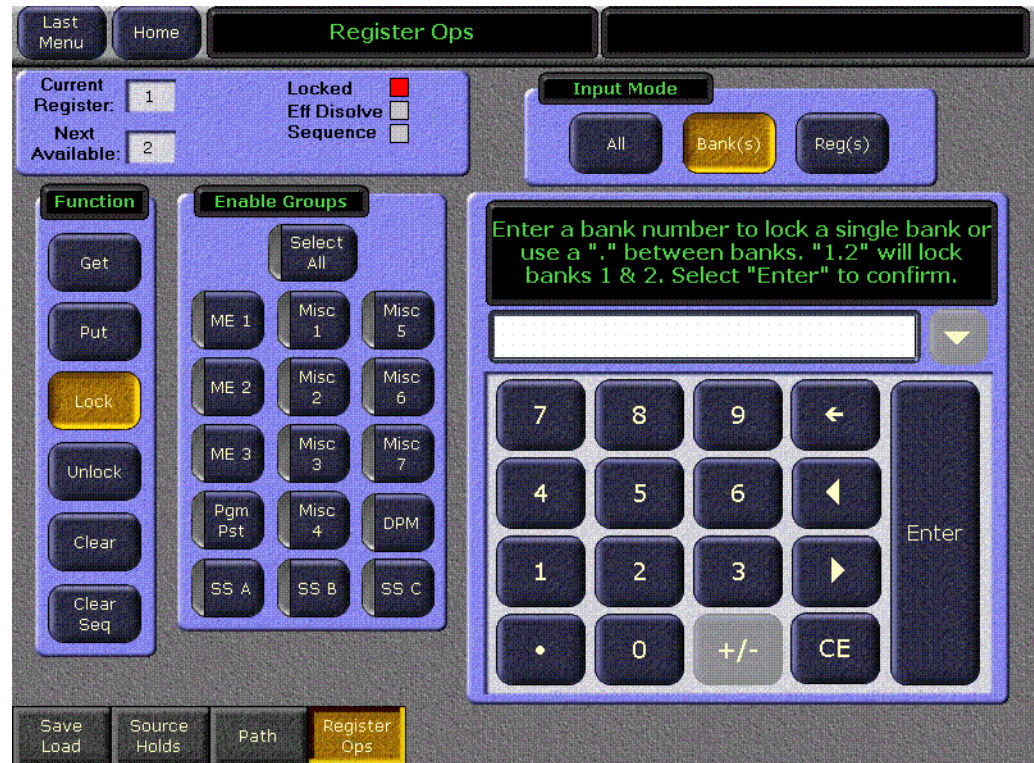
Figure 3. E-MEM Register Operations Menu, Lock Selected
