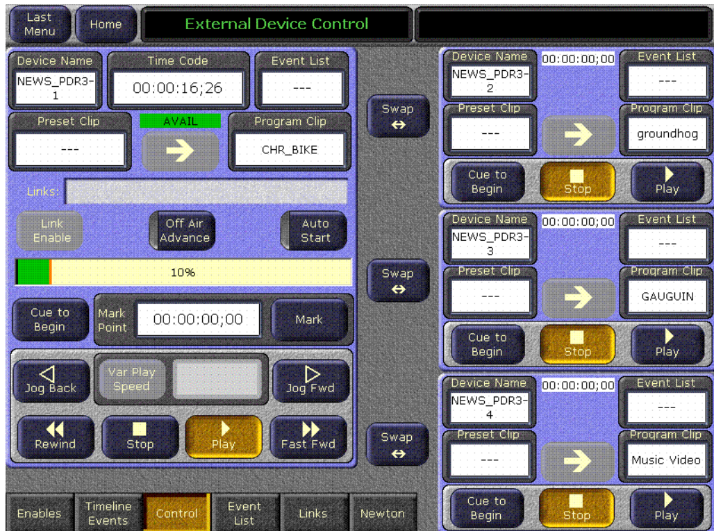
Figure 39. External Device Control Menu
