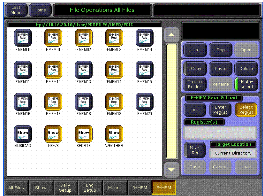
Figure 24. Multiselect Button Allows Selection of Multiple Files
