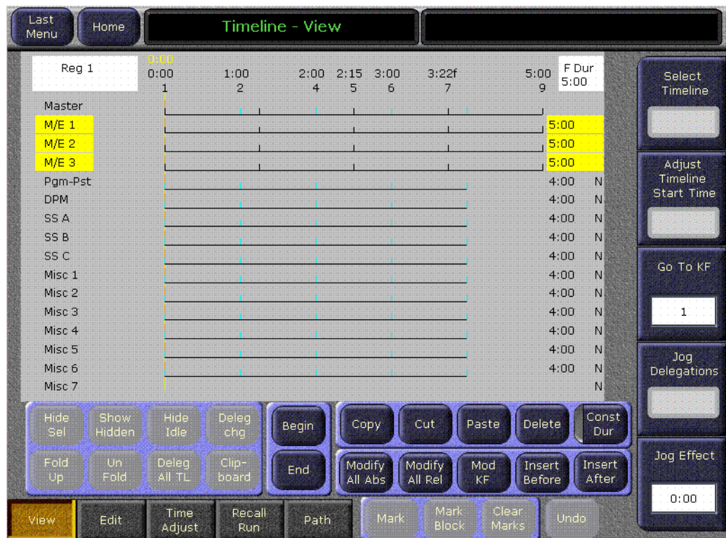
Figure 8. Timeline - Time Adjust Menu, Forced Duration of Individual Levels
