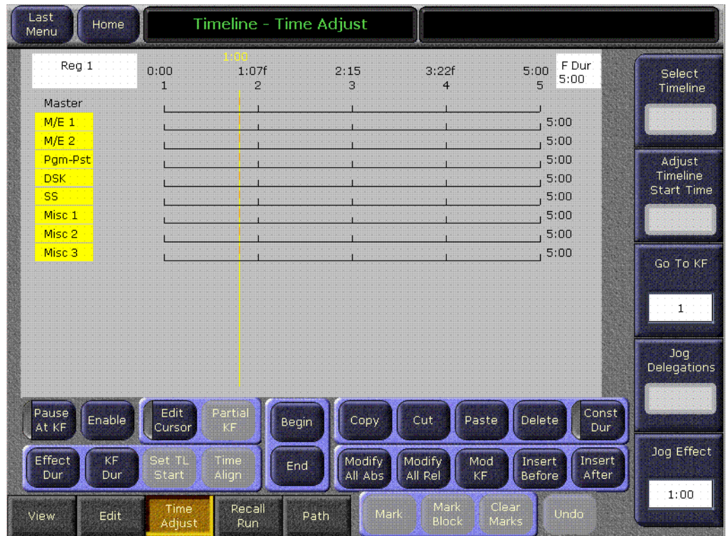
Figure 6. Timeline - Time Adjust Menu, Forced Duration
