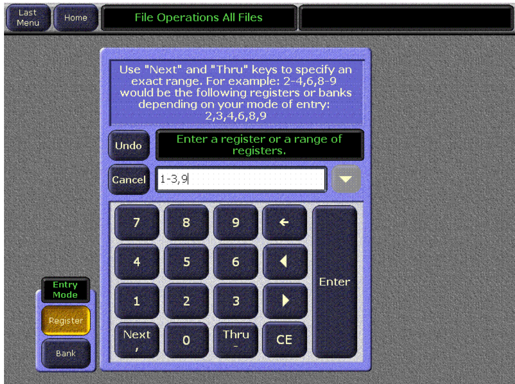
Figure 15. File Operations Register Entry Window
