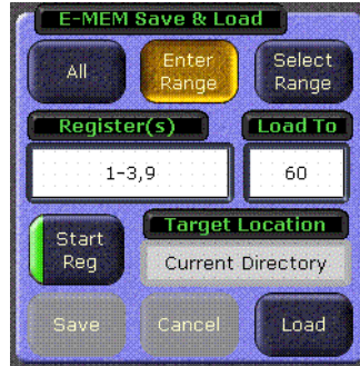
Figure 19. File Operations Register(s) and Load To Text Entry Boxes
