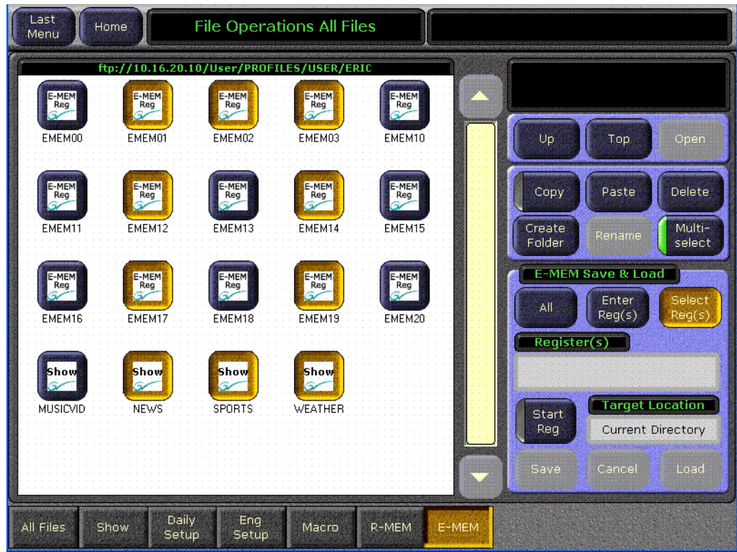
Figure 20. Multiselect Button Allows Selection of Multiple Files
