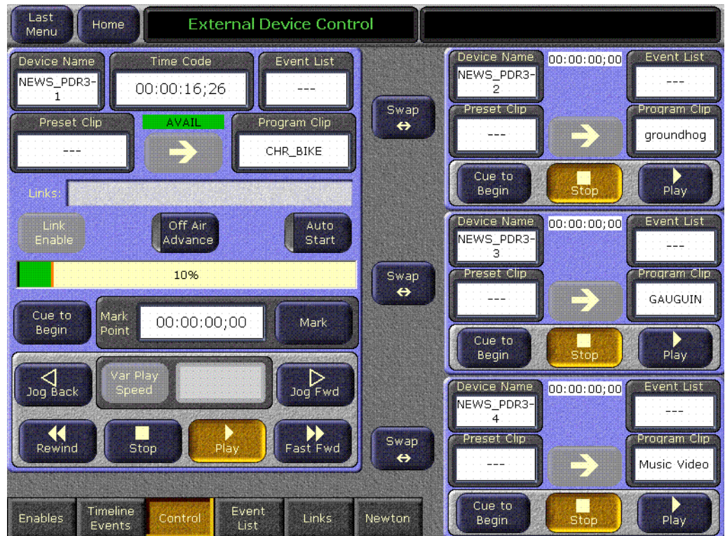
Figure 33. External Device Control Menu
