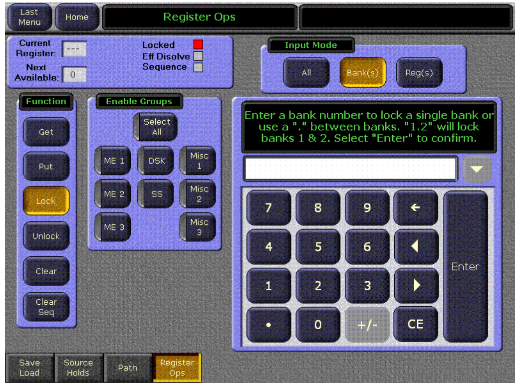
Figure 3. E-MEM Register Operations Menu, Lock Selected
