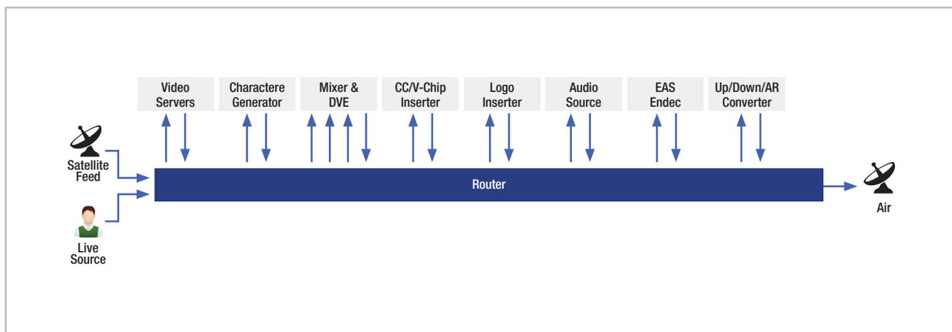
Figure 2 – Conventional Broadcast Transmission Chain
